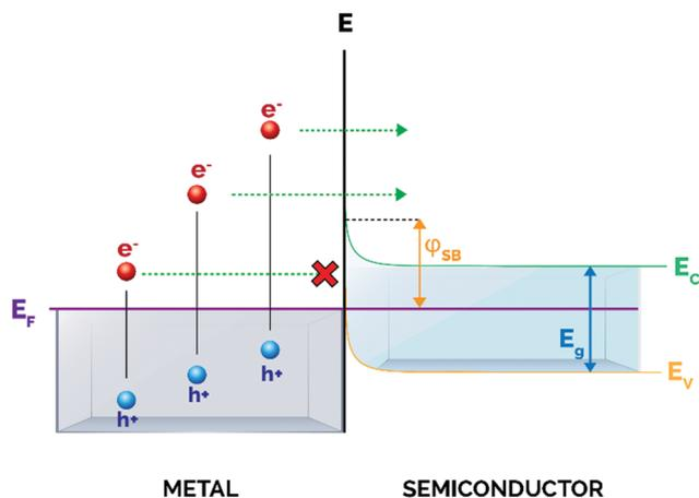
Fig. 3 Schematic illustration of the metal/semiconductor Schottky barrier. Upon excitation, only hot electrons with enough energy can surpass the Schottky barrier ( $\phi_{\text{SB}}$ ) and transfer into the conduction band of the semiconductor.
