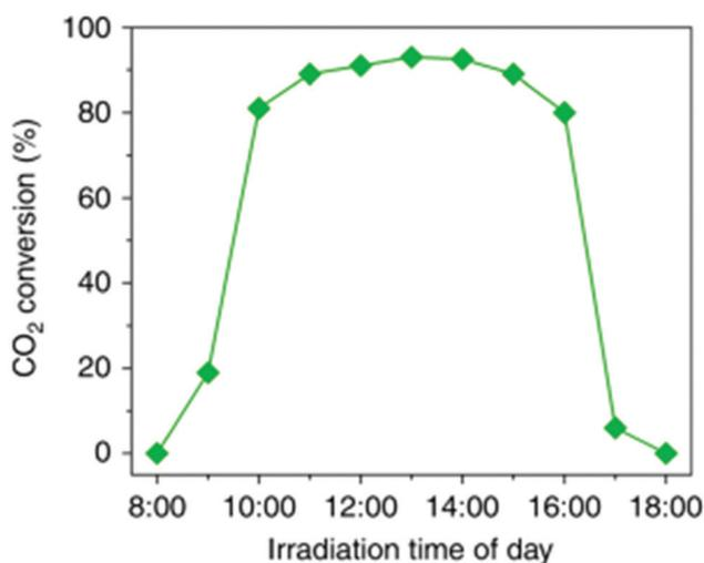
Fig. 12 Photo-thermal CO<sub>2</sub> conversion using SA Ni/Y<sub>2</sub>O<sub>3</sub> nanosheets with a selective light absorber-assisted photo-thermal system as a function of time. Experiment carried out on June 30, 2018 from 8:00 to 18:00 in Baoding, Hebei, China. Reproduced with permission from ref. 207. Copyright (2019) Springer Nature.
