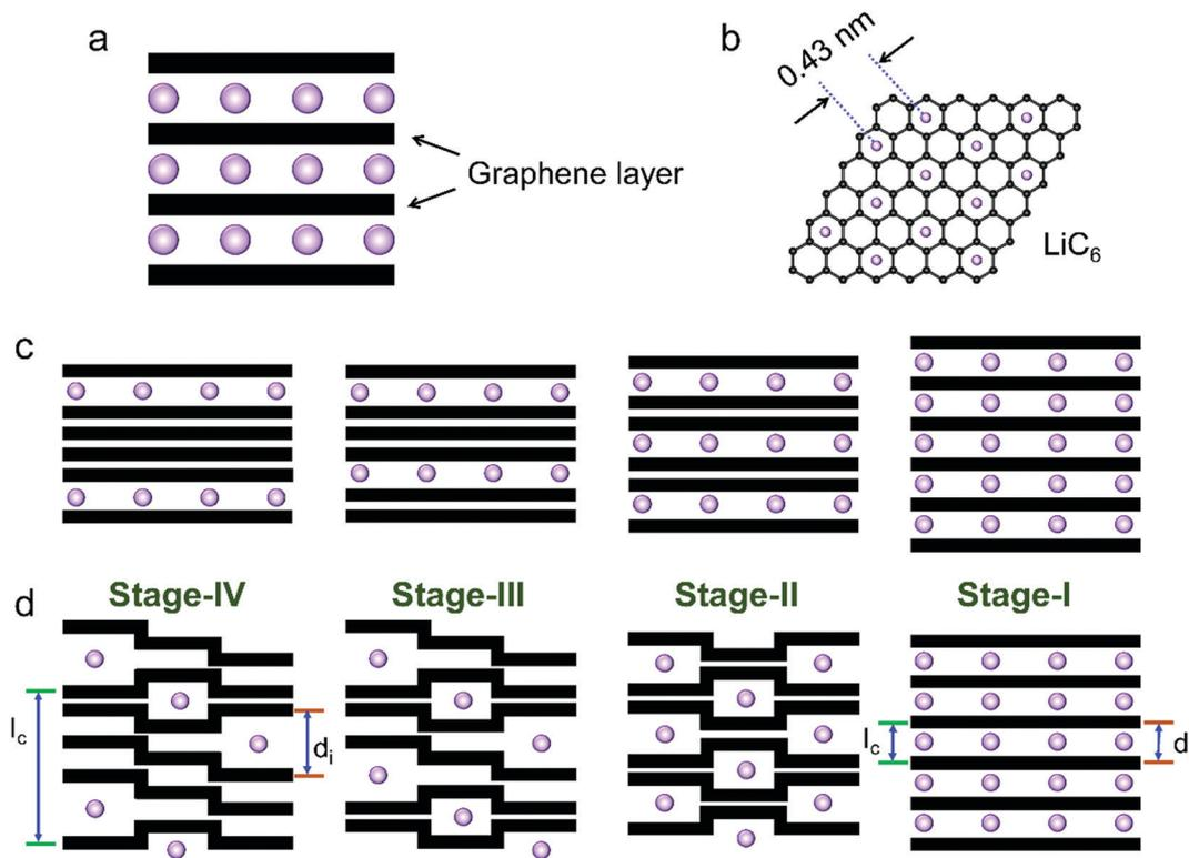
Fig. 4 Schematic illustration of (a) Li-intercalated graphite and (b) the formed  $\text{LiC}_6$  structure. Two models of the stage formation process during Li<sup>+</sup> intercalation into graphite: (c) Rüdorff model and (d) Daumas-Hérol model.
