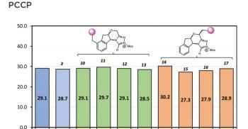
Fig. 7 The Gibbs free energy barriers and reaction free energies at 298 K for decarboxylation of 5. The uncatalyzed pathway is compared with that catalysed by the original NHC·H+ 3 and its various modified versions shown in Scheme 2. The units are in kcal mol<sup>-1</sup>.
