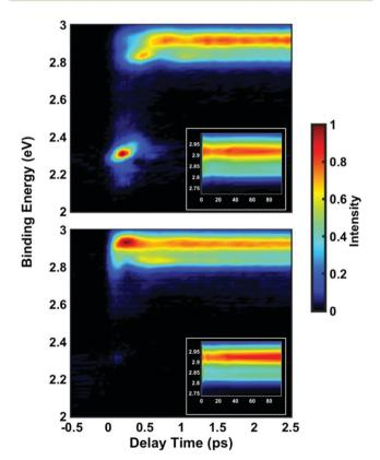
Fig. 2 Time-resolved photoelectron spectra of NMP upon 212 nm (top) and 229 nm (bottom) excitation. The insets show the 3s state signals up to 100 ps. The color represents the normalized intensity in arbitrary units as indicated by the color bar.
