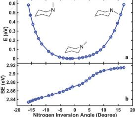
**Fig. 4** The computed potential energy of NMP in the 3s Rydberg state as a function of the nitrogen inversion angle (the definition of this angle is shown in ESI†), (a), and the corresponding binding energy of the 3s Rydberg state (b).
