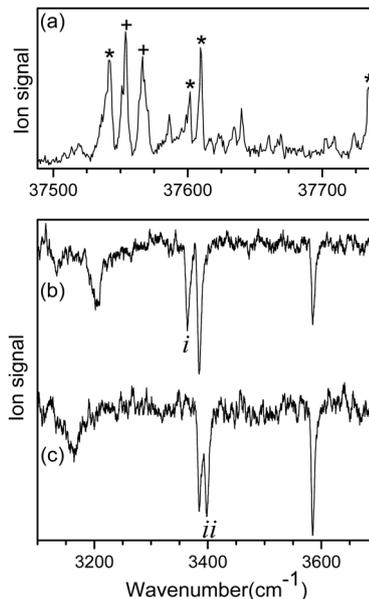
Fig. 1 (a) UVPD spectrum of L-H<sup>+</sup>PheAla near the origin band of the S<sub>0</sub>-S<sub>1</sub> transition obtained by monitoring the sum of fragment signals at  $m/z$  145 and 149. IR ion-dip spectra obtained by fixing a UV probe laser at the vibronic bands labeled as (b) \* and (c) +, respectively.
