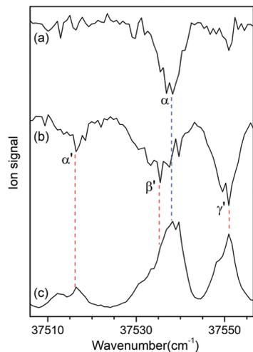
Fig. 3 UV-UV HB spectra of conformers (a) I and (b) II obtained by fixing the UV pump laser at the bands  $\beta$  and  $\gamma'$  in Fig. 2, respectively. (c) UVPD spectrum of L-H<sup>+</sup>PheAla shown for comparison.
