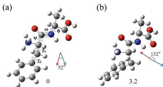
**Fig. 7** Structures of conformers (a) I and (b) II of L-H<sup>+</sup>PheAla optimized at the CAM-B3LYP/6-311++G(d,p) level. The dihedral angles of the structures are labeled as  $\psi$ ,  $\omega$ ,  $\phi$ ,  $\chi_1$ , and  $\chi_2$ . The red and blue arrows represent  $\mu$  and  $m$ , respectively. The numbers at the bottom are the relative energies of the conformers in kJ mol<sup>-1</sup>.
