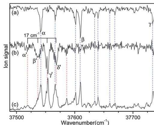
Fig. 2 IR-UV HB spectra obtained by fixing an IR pump laser at vibrational bands (a) *i* and (b) *ii* in the IR ion-dip spectra in Fig. 1. (c) UVPD spectrum of L-H<sup>+</sup>PheAla shown for comparison.
