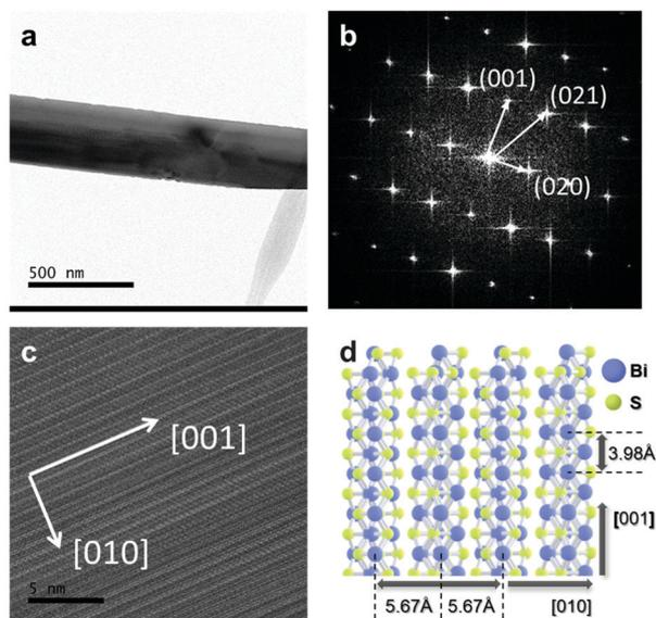
Fig. 4 Structure analysis of  $\text{Bi}_2\text{S}_3$ . (a) TEM image of  $\text{Bi}_2\text{S}_3$  on a TEM grid, (b) SAED patterns of single crystalline  $\text{Bi}_2\text{S}_3$ , (c) HRTEM image of anisotropic  $\text{Bi}_2\text{S}_3$  structure, and (d) schematic illustration of  $\text{Bi}_2\text{S}_3$  crystal structure.
