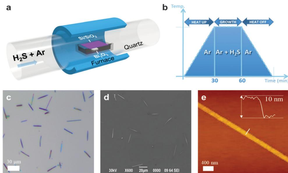
**Fig. 1** The synthesis method of Bi<sub>2</sub>S<sub>3</sub> and its characterization. (a) Schematic illustration of experimental set-up of Bi<sub>2</sub>S<sub>3</sub>, (b) diagram of synthesis process of Bi<sub>2</sub>S<sub>3</sub>, (c) OM image of as-grown Bi<sub>2</sub>S<sub>3</sub>, (d) SEM image of as-grown Bi<sub>2</sub>S<sub>3</sub>, and (e) AFM image and height profile of as-grown Bi<sub>2</sub>S<sub>3</sub>.
