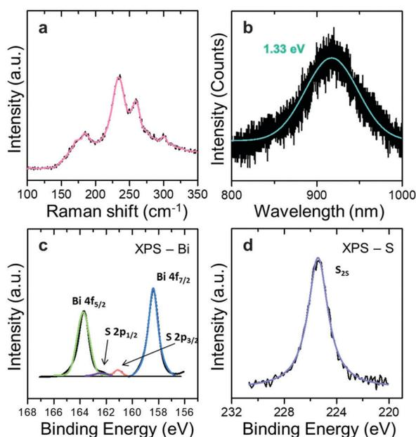
Fig. 2 Characterization of optical properties and stoichiometry analysis of  $\text{Bi}_2\text{S}_3$ . (a) Raman spectrum of  $\text{Bi}_2\text{S}_3$ , (b) PL spectrum of  $\text{Bi}_2\text{S}_3$ , (c) XPS spectrum of Bi 4f peaks and S 2p peaks, and (d) XPS spectrum of S 2s peaks.
