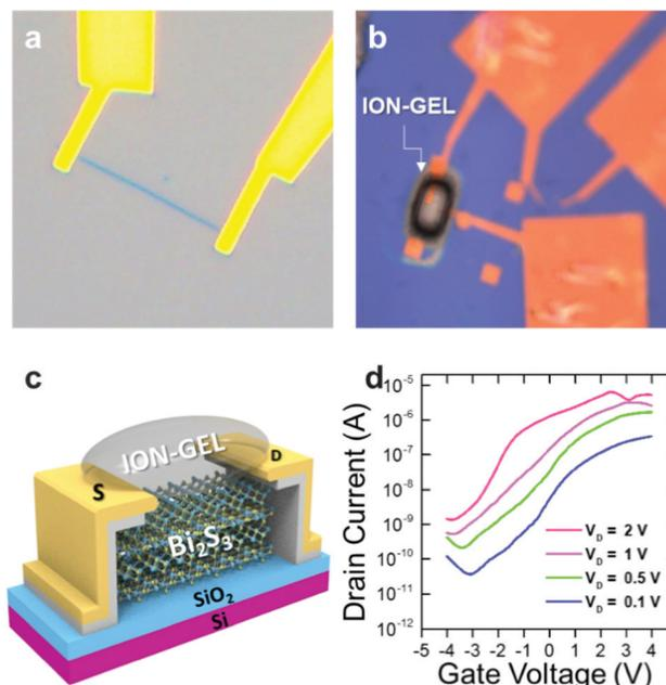
Fig. 5 Electronic properties of  $\text{Bi}_2\text{S}_3$ : (a) OM image of FET based on as-grown  $\text{Bi}_2\text{S}_3$ , (b) OM image of the ion-gel gated transistor of  $\text{Bi}_2\text{S}_3$ , (c) schematic diagram of ion-gel gated  $\text{Bi}_2\text{S}_3$  FET, (d) transfer characteristics of  $\text{Bi}_2\text{S}_3$  transistor.
