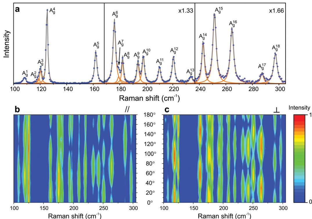
Fig. 7 Characteristic Raman spectrum of the triclinic ReSe<sub>2</sub>; (a) Raman spectrum of a monolayer ReSe<sub>2</sub> showing the 18 A<sub>g</sub> modes predicted by group theory. Typical angle-resolved Raman map of ReSe<sub>2</sub> in the (b) parallel (//) and (c) crossed (⊥) configurations. The spectra and mapping were collected with a 2.33 eV laser energy. Adapted with permission from ref. 19.
