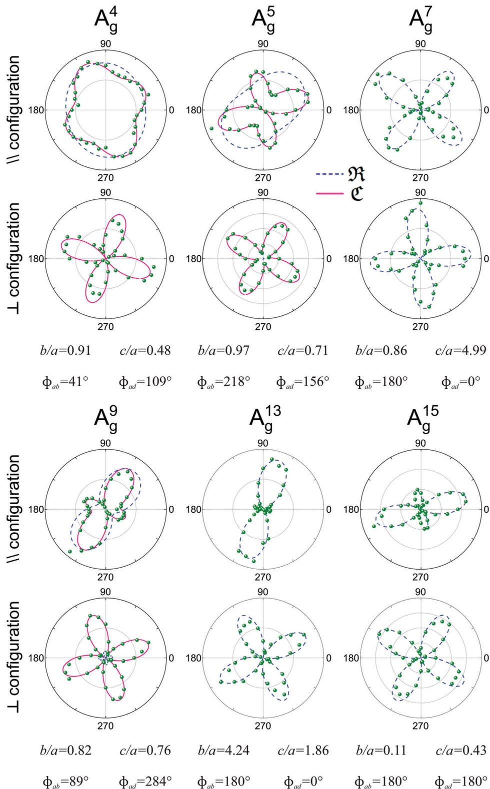
**Fig. 8** Typical Raman polar plots of a monolayer triclinic  $\text{ReSe}_2$ . Angular dependence of the intensities of 6  $A_g$  modes in the parallel ( $\parallel$ ) and crossed ( $\perp$ ) configurations for an exfoliated monolayer  $\text{ReSe}_2$  collected using an excitation energy of 2.33 eV. The corresponding tensor element ratios and phase differences extracted from the fitting process are also shown. Adapted with permission from ref. 19.
