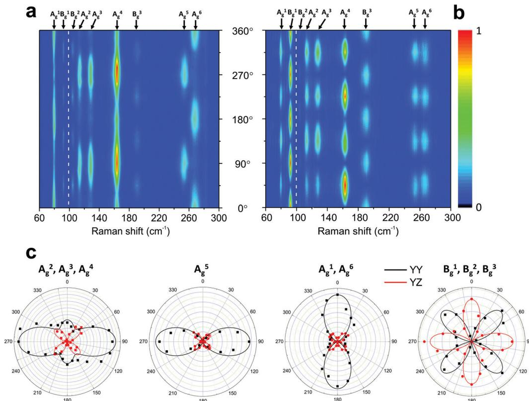
Fig. 6 Typical angle-resolved Raman map of a monoclinic 1T'-MoTe<sub>2</sub>. Raman map in the (a) parallel (||) and (b) crossed (⊥) polarization configurations. (c) Angular dependence of the intensities of the 1T'-MoTe<sub>2</sub> peaks shown in (a) and (b). The angle-resolved Raman map was constructed using two excitation energies: 1.96 eV (below 100 cm<sup>-1</sup>) and 2.33 nm (above 100 cm<sup>-1</sup>). Adapted with permission from ref. 50.
