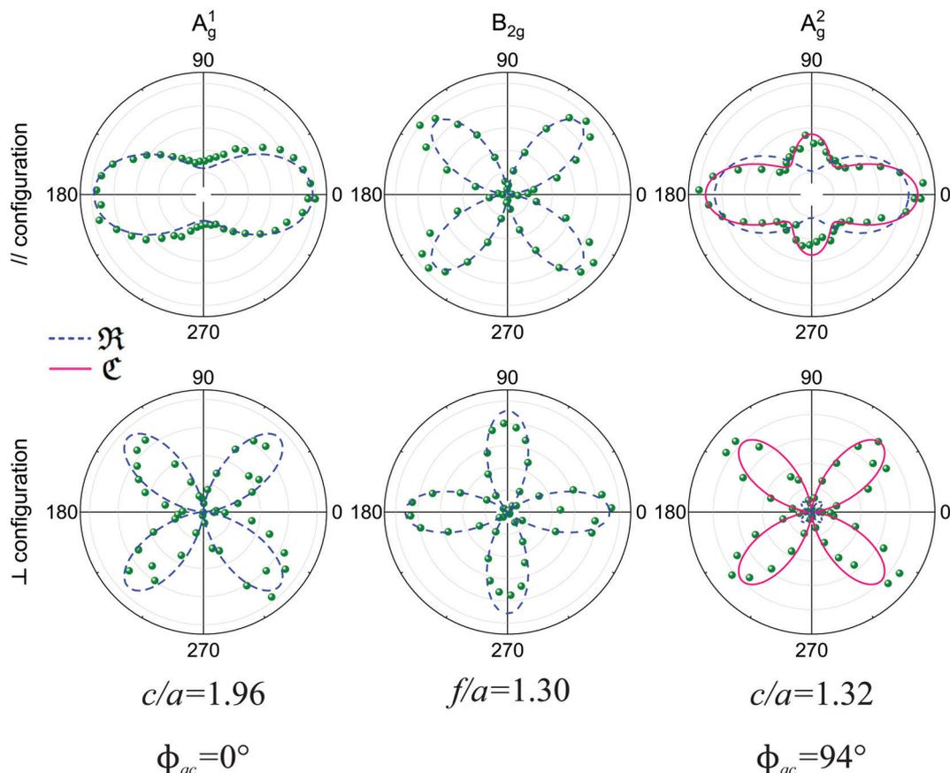
Fig. 5 Angle-resolved Raman response of the orthorhombic black phosphorus. Angular dependence of the intensities of the  $A_g^1$ ,  $B_{2g}$  and  $A_g^2$  modes in the parallel ( $\parallel$ , top panel) and crossed ( $\perp$ , bottom panel) polarization configurations for an exfoliated BP flake for an excitation energy of 2.33 eV. The corresponding tensor element ratios and phase differences extracted from the fitting process are also shown. Adapted with permission from ref. 21.
