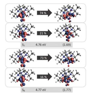
Fig. 7 Natural transition orbitals (NTOs) of the two dominant singlet states  $S_7$  at 4.76 eV (260.5 nm) and  $S_8$  at 4.77 eV (259.9 nm) with the corresponding weights of the NTO pair given inside the arrow (TD-DFT B3LYP-D3(BJ)/def2-SVP; implicit acetonitrile); labelling includes state, excitation energy and PR<sub>NTO</sub> in parenthesis (the participation ratio indicates how many NTO pairs are representative for a state).
