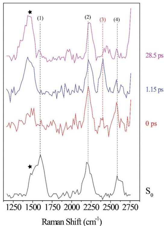
Fig. 5 ODIBO FSRS spectra after 321 nm excitation at 0, 1.15 and 28.5 ps delay-times with peaks at 2206, 2399 and 2578 cm<sup>-1</sup> at 0 ps labeled (2), (3), and (4), respectively. The ground state spectrum (black) without actinic excitation is also provided with 1601, 2206 and 2582 cm<sup>-1</sup> peaks labeled (1), (2) and (4) respectively. The black stars denote a methanolic peak at 1483 cm<sup>-1</sup>.
