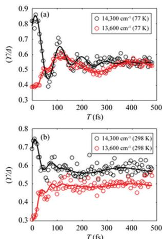
**Fig. 3** (a and b) Temporal evolution of  $\gamma/\Delta_{\text{reph}}$  at  $14\,300\text{ cm}^{-1}$  (black empty dots) and  $13\,600\text{ cm}^{-1}$  (red empty dots), which correspond to dashed lines in Fig. 2a and b, and their fits using two damped cosine functions and an exponential decay (solid lines of their corresponding colors) at (a) 77 K and (b) 298 K.
