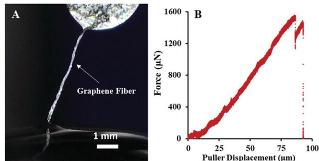
Fig. 3 Macroscale graphene fiber tested in uniaxial tension. (A) Optical image of graphene fiber ( $A_{\text{graphene}} = 3.18 \mu\text{m}^2$ ,  $L_{\text{fiber}} = 2952 \mu\text{m}$ ). (B) Force–displacement plot of uniaxial tensile test (puller displacement rate  $r_p = 0.50 \mu\text{m s}^{-1}$ ). This fiber exhibited brittle fracture, with a tensile strength of 0.475 GPa.
