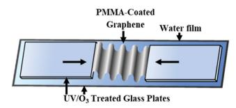
Fig. 1 Schematic of folding process for PMMA-coated graphene in an accordion-like pattern. Glass plates were treated with UV/O<sub>3</sub> prior to use. Wrinkles formed in the graphene sheet during compression along the width of the graphene sheet and remained folded as the sheet was compressed further
