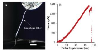
Fig. 3 Macroscale graphene fiber tested in uniaxial tension. (A) Optical image of graphene fiber ( $A_{graphene} = 3.18 \mu m^2$ ,  $L_{fiber} = 2952 \mu m$ ). (B) Forcedisplacement plot of uniaxial tensile test (puller displacement rate  $r_p = 0.50 \,\mu\text{m s}^{-1}$ ). This fiber exhibited brittle fracture, with a tensile strength of 0.475 GPa.
