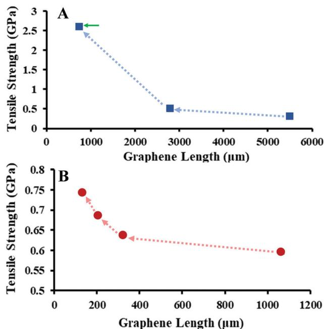
Fig. 5 Breaking strength of graphene fibers as a function of fiber length. Dotted arrows indicate order of sequential uniaxial tensile tests on the same fibers with  $A_{\text{graphene}} = 3.2 \mu\text{m}^2$  (A) and  $A_{\text{graphene}} = 5.2 \mu\text{m}^2$ . (B) Green arrow indicates a measurement where ductile fracture behavior was observed during tensile testing.
