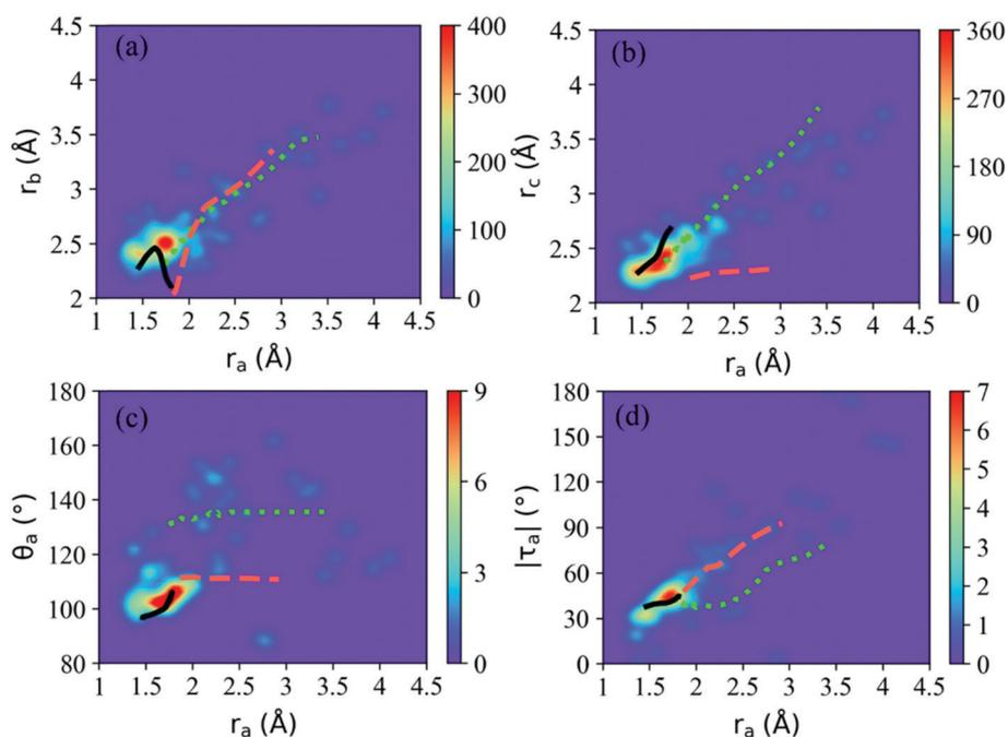
Fig. 6 Distribution of the important geometric parameters at the first  $S_1$  to  $S_0$  hops within 120 fs. In all panels, the green dotted line, orange dashed line, and black solid line mark the  $\text{CI}_{10}$ -seam-I,  $\text{CI}_{10}$ -seam-II, and  $\text{CI}_{10}$ -seam-III, respectively.
