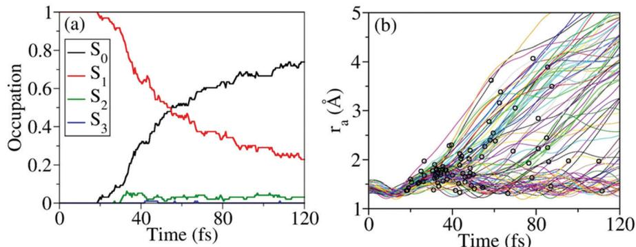
Fig. 5 Time-dependent (a) average fractional occupation and (b)  $r_a$  value of several trajectories simulated in the nonadiabatic dynamics starting from  $S_1$  at the XMS(4)-CASPT2(12,9)/def2-SVPD level. Black circles mark the  $S_1$  to  $S_0$  hops. After 120 fs, the electronic structure calculations of several trajectories may not be converged at random steps. Thus the overall population dynamics is only shown up to 120 fs.
