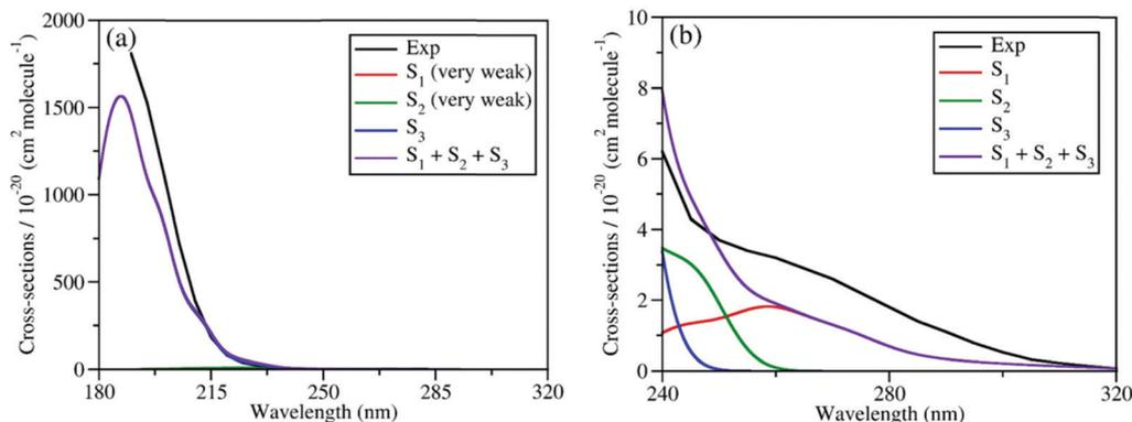
Fig. 2 Comparison of experimental and simulated UV absorption spectra of  $\text{CH}_3\text{ONO}_2$ : (a) from 180 nm to 320 nm; (b) from 240 nm to 320 nm. The theoretical spectra were simulated at XMS(4)-CASPT2(12,9)/def2-SVPD level. The experimental spectra in (a) and (b) were taken from previous works.<sup>6,27</sup> The intensities of absorption bands shown in (a) and (b) differ by several magnitudes.
