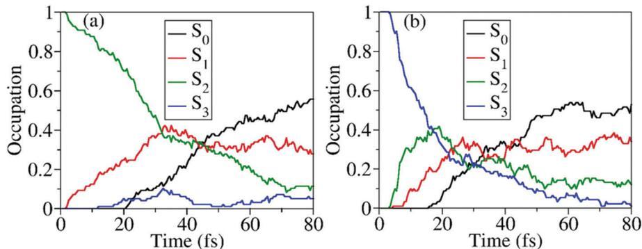
Fig. 8 Time-dependent average fractional occupations of adiabatic electronic states in nonadiabatic dynamics: (a) initiated from  $S_2$ ; (b) initiated from  $S_3$ . After 80 fs, the electronic structure calculations of several trajectories may not be converged at random steps. Thus the overall population dynamics is only shown up to 80 fs.
