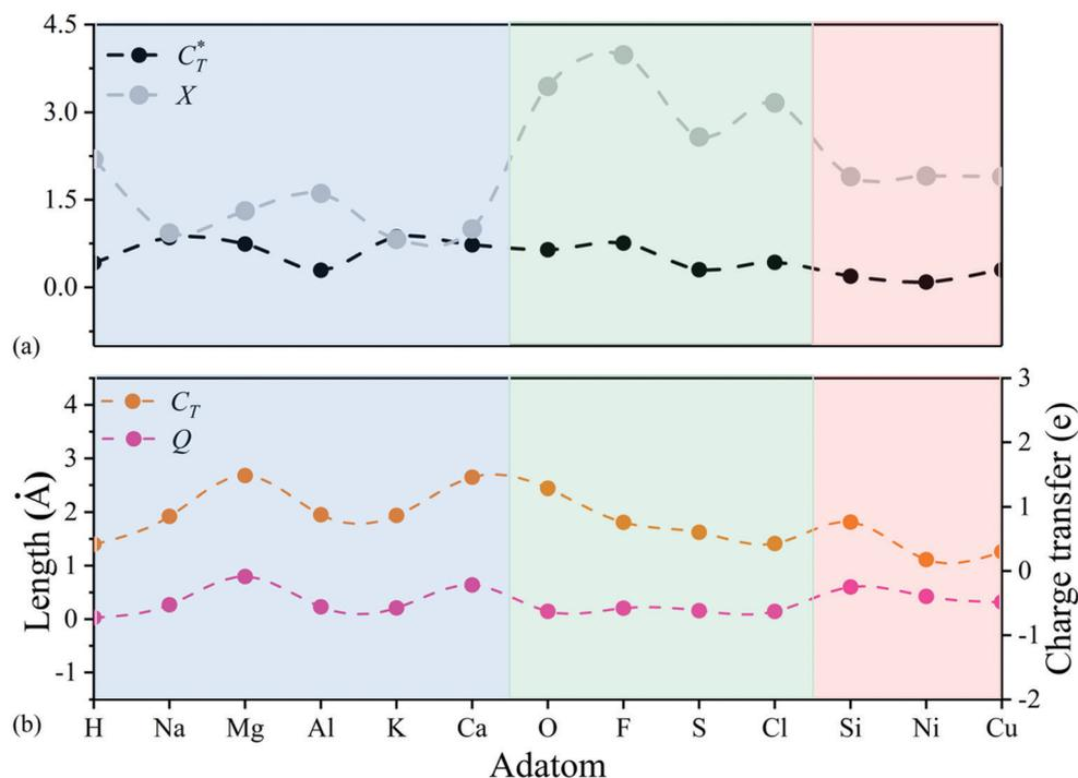
**Fig. 4** (a) Charge transfer capability ( $C_T^*$ , dashed black curve) and electronegativity ( $X$ , dashed grey curve) for different adatoms. (b) Comparison between the distortion magnitude of N<sub>2</sub>P<sub>6</sub> structure ( $Q$ , dashed rose curve) and the charge transfer of adatoms ( $C_T$ , dashed orange curve). The adsorption type of T<sub>N</sub>, T<sub>P</sub>, H<sub>PP</sub> are represented by light blue, green and red area, respectively.
