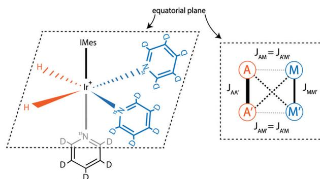
**Fig. 1** Structure of the iridium SBRE complex; molecular hydrogen and the substrate (with two  $Py$  ligands in equatorial positions, and a third  $Py$  in an axial position) are indicated. The spin system of the SABRE complex is also shown, here modelled as an  $AA'MM'$  system (A-spins stand for the  $pH_2$  protons and M-spins belong to the  $^{15}N$  nuclei of the two equatorial  $Py$  ligands).
