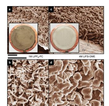
Fig. 13 Scanning electron microscope images of the morphologies of Li metal after plating on Cu substrates in different electrolytes. (a and b) 1 mol dm $^{-3}$  LiPF $_6$ /PC. (c and d) 4 mol dm $^{-3}$  LiFSA/DME (G1). The current density was 1.0 mA cm<sup>-2</sup> and the deposition time was 1.5 h. The diameter of the Cu substrate shown in the inset of (a and c) was 2 cm. Scale bar, 10 µm. Reprinted with permission from ref. 52 Copyright 2015 Nature Publishing Group.
