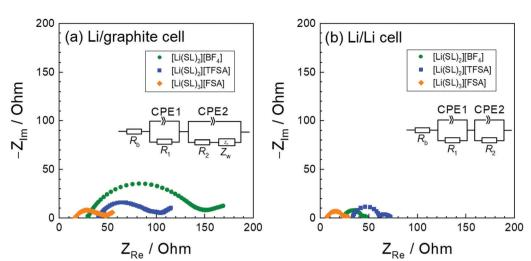
Fig. 15 Nyquist plots of (a) Li/graphite cells at a 67% state of charge in the 3rd cycle and (b) Li/Li symmetric cells containing electrolytes of [Li(SL)<sub>2</sub>][BF<sub>4</sub>], [Li(SL)<sub>2</sub>][TFSA], and [Li(SL)<sub>3</sub>][FSA] at 30 °C. The geometrical areas of the Li-metal and graphite electrodes were both 2.0 cm<sup>2</sup>
