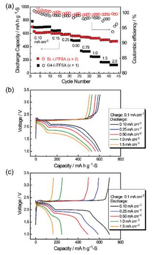
Fig. 18 (a) Discharge capacity and Coulombic efficiency at different discharge current densities, and charge and discharge curves of the cells using the concentrated electrolytes, (b) [Li(SL)2][TFSA] and (c) [Li(G4)<sub>1</sub>][TFSA]. Reprinted with permission from ref. 39 Copyright 2019 American Chemical Society
