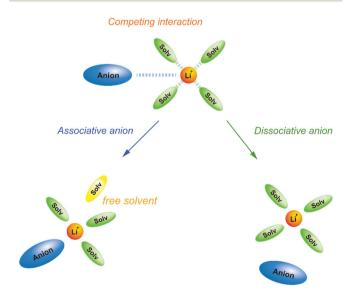
Fig. 5 Schematic illustration for the effect of Lewis basicity of anion on the solvation structure in highly concentrated electrolytes.
