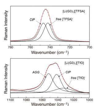
Fig. 6 Raman spectra of [Li(G3)<sub>1</sub>][TFSA] in the range 700-780 cm<sup>-1</sup> (top, CF<sub>3</sub> bending mode) and of [Li(G3)<sub>1</sub>][TfO] in the range 1000-1100 cm<sup>-1</sup> (bottom, SO<sub>3</sub> stretching mode) at 60 °C. Reprinted with permission from ref. 58 Copyright 2014 American Chemical Society.
