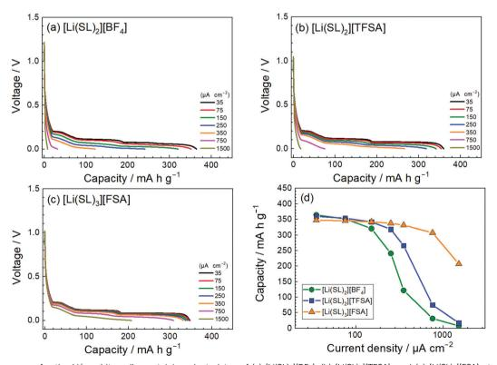
Fig. 14 Charge curves for the Li/graphite cells containing electrolytes of (a) [Li(SL)<sub>2</sub>][BF<sub>4</sub>], (b) [Li(SL)<sub>2</sub>][TFSA], and (c) [Li(SL)<sub>3</sub>][FSA] at various current densities at 30 °C. (d) Charge capacities of the cells as functions of current density. Following each charge measurement, the cell was fully discharged at the low current density of 35  $\mu$ A cm<sup>-2</sup>.
