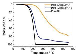
Fig. 7 Thermogravimetric curves of NaFSA/SL electrolytes at a heating rate of 10 °C min<sup>-1</sup>. Reprinted with permission from ref. 34 Copyright 2020 American Chemical Society.
