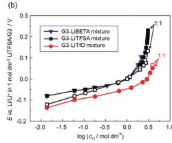
Fig. 3 Plots of the Li/Li<sup>+</sup> electrode potential against a common logarithm of the Li salt concentration in (a) G4 (tetraglyme), G3 (triglyme), G2 (diglyme), G1 (monoglyme), and THF-LiTFSA mixtures; (b) G3-LiTFO, -LiTFSA, and -LiBETA mixtures at 30 °C. Reference electrode was Li/Li<sup>+</sup> in 1 mol dm<sup>-3</sup> LiTFSA/ G3. (b) was reprinted with permission from ref. 59 Copyright 2015 PCCP Owner Societies.
