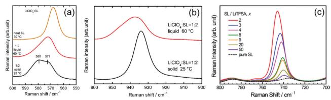
Fig. 9 Raman spectra of (a) scissoring mode of the  $SO_2$  group of SL and (b) Cl-O symmetric stretch vibration mode of  $ClO_4^-$  in the [Li(SL)<sub>2</sub>](ClO<sub>4</sub>] solvate. Reprinted with permission from ref. 31 Copyright 2018 American Chemical Society. (c) Raman spectra of the S-N stretching vibration mode of TFSA<sup>-</sup> anion in the LiTFSA/SL binary mixtures. Reprinted with permission from ref. 39 Copyright 2019 American Chemical Society.
