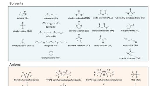
Fig. 2 Chemical structures and abbreviations of the various solvents and anions
