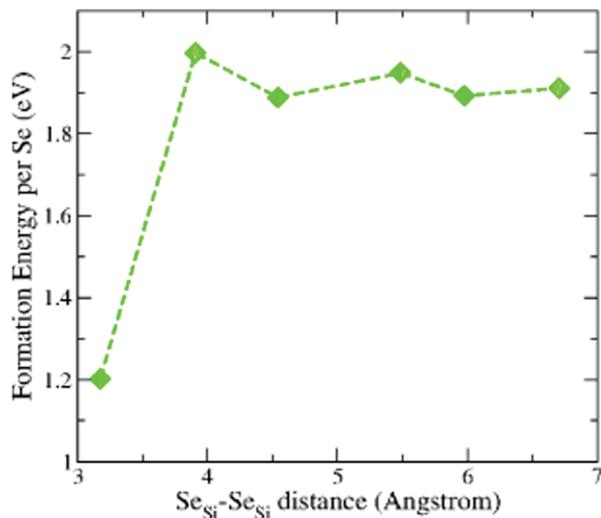
Fig. 11 Formation energy (per atom) of a couple of Se substitutional impurities in Se hyperdoped Si,  $\text{Si}_{1-x}\text{Se}_x$ , at  $x = 0.93$  at%. One Se is placed at the  $n$ -neighbour shells ( $\text{NN}^n$ ,  $n = 1, 2, \dots, 6$ ) surrounding the other Se. Se–Se distance refers to relaxed positions and increases according to the increasing shell number  $n$ . Dashed line is a guide for the eye.
