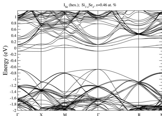
Fig. 8 Electronic bandstructure of Se hyperdoped Si,  $\text{Si}_{1-x}\text{Se}_x$ , for Se interstitial,  $\text{I}_{\text{Se}}$ , in tetrahedral (top panel) and hexagonal position (bottom panel) at  $x = 0.461$  at%. The zero of the energy scale corresponds to the Fermi energy.
