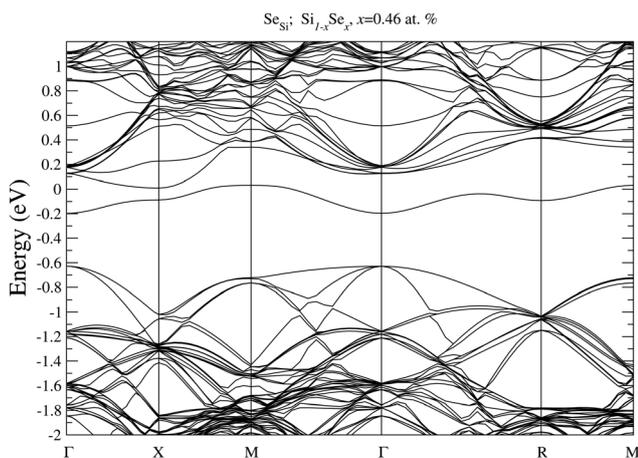
Fig. 5 Electronic bandstructure of Se hyperdoped Si,  $\text{Si}_{1-x}\text{Se}_x$ , for single  $\text{Se}_{\text{Si}}$  at  $x = 0.46$  at%. The zero of the energy scale corresponds to the Fermi energy.
