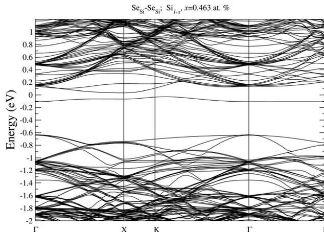
Fig. 7 Electronic bandstructure of Se hyperdoped Si,  $\text{Si}_{1-x}\text{Se}_x$ , for substitutional  $\text{Se}_{\text{Si}}\text{-Se}_{\text{Si}}$  dimer at  $x = 0.463$  at%. The zero of the energy scale corresponds to the Fermi energy.
