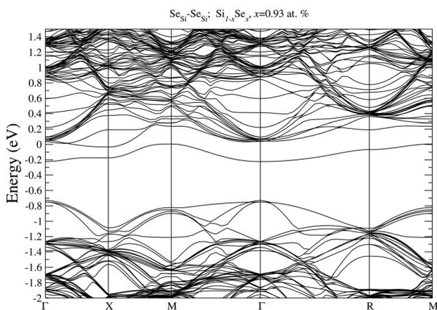
Fig. 6 Electronic bandstructure of Se hyperdoped Si  $\text{Si}_{1-x}\text{Se}_x$ , for  $\text{Se}_{\text{Si}}\text{-Se}_{\text{Si}}$  dimer at  $x = 0.93$  at%. The zero of the energy scale corresponds to the Fermi energy.
