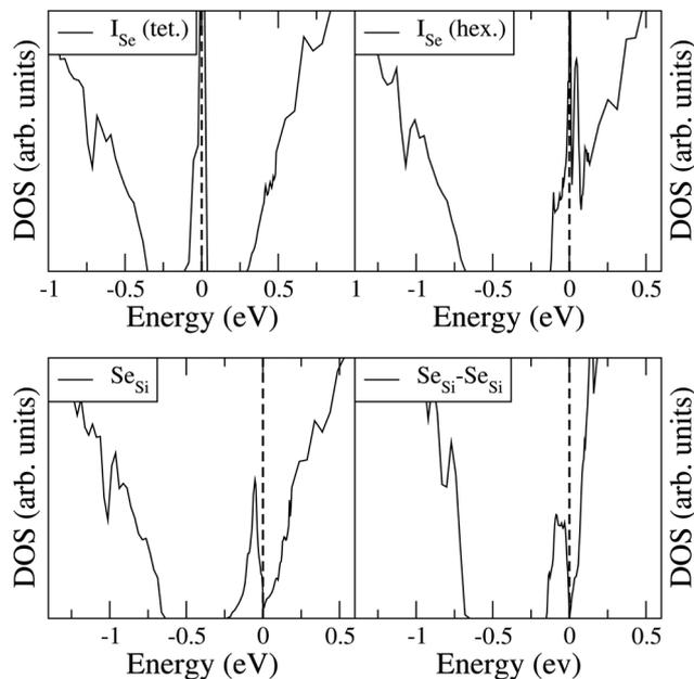
Fig. 3 Electronic DOS of  $\text{Si}_{1-x}\text{Se}_x$  for Se interstitial in the tetrahedral and hexagonal positions at  $x = 0.461$  at%, and for substitutional single  $\text{Se}_{\text{Si}}$  and  $\text{Se}_{\text{Si}}-\text{Se}_{\text{Si}}$  dimers at  $x = 0.463$  at%.
