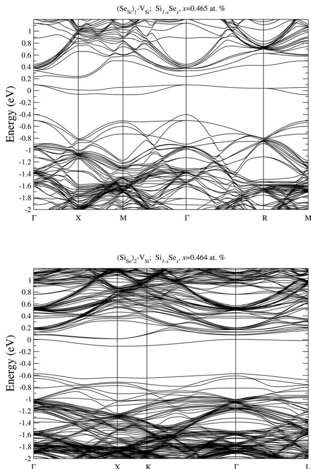
Fig. 9 Electronic bandstructure of Se hyperdoped Si,  $\text{Si}_{1-x}\text{Se}_x$ , for  $(\text{Se}_{\text{Si}})_1\text{-V}_{\text{Si}}$  at  $x \approx 0.465$  at% (top panel), and for  $(\text{Se}_{\text{Si}})_2\text{-V}_{\text{Si}}$  at  $x \approx 0.464$  at% (bottom panel). The zero of the energy scale corresponds to the Fermi energy.
