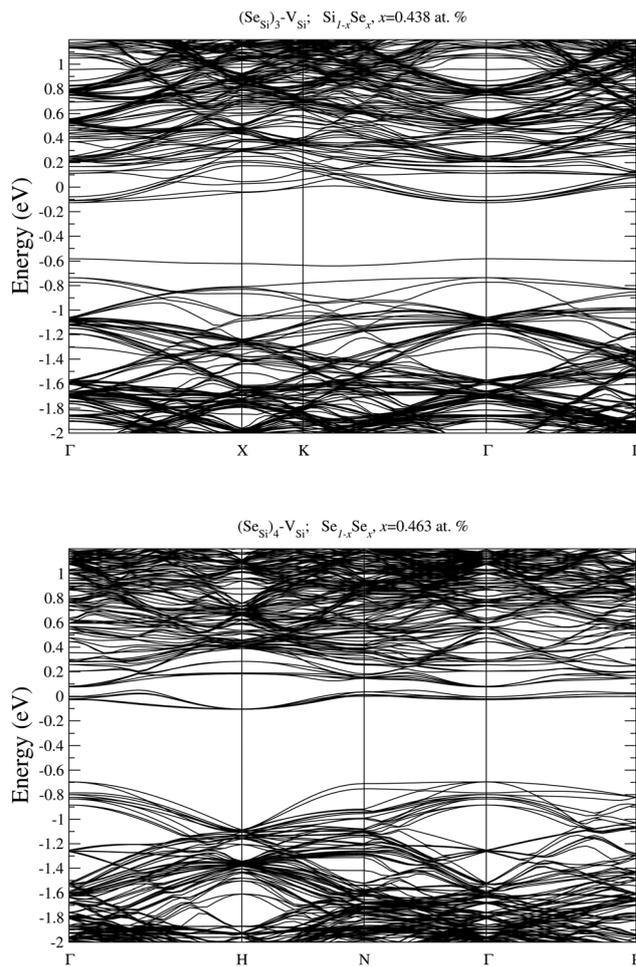
Fig. 10 Electronic bandstructure of Se hyperdoped Si,  $\text{Si}_{1-x}\text{Se}_x$ , for  $(\text{Se}_{\text{Si}})_3\text{-V}_{\text{Si}}$  at  $x \approx 0.438$  at% (top panel), and for  $(\text{Se}_{\text{Si}})_4\text{-V}_{\text{Si}}$  at  $x \approx 0.463$  at% (bottom panel). The zero of the energy scale corresponds to the Fermi energy.
