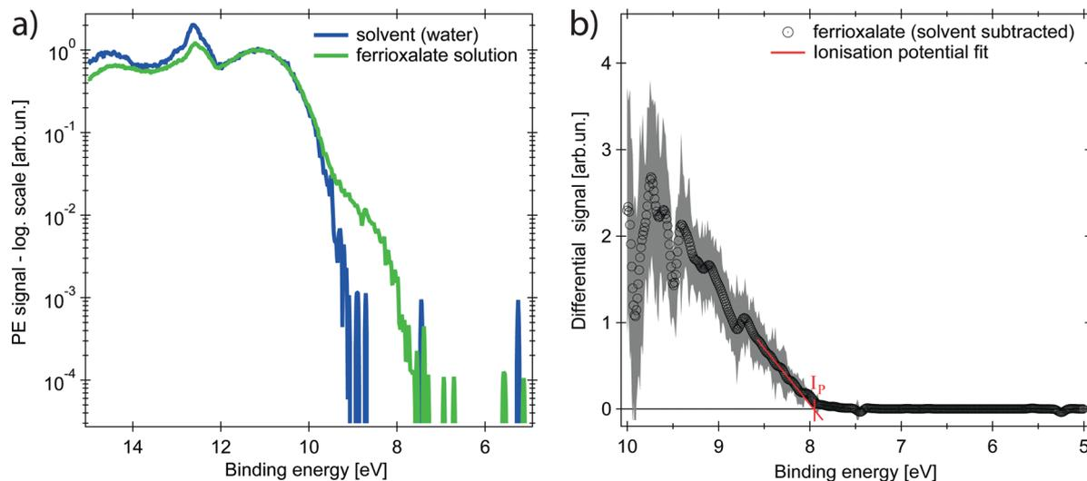
Fig. 2 Steady-state photoelectron (PE) spectra ( $h\nu = 37.2$  eV). (a) Solution of aqueous ferrioxalate (green, 0.5 molar) and pure water solvent (blue), plotted on a logarithmic scale and normalised to the  $1b_1$  band of water at 11.16 eV. (b) Differential spectrum showing the ferrioxalate HOMO band only, whose ionisation potential is  $I_p = (7.9 \pm 0.2)$  eV. Experimental uncertainty of  $2\sigma$  as shaded grey area around the trace.
