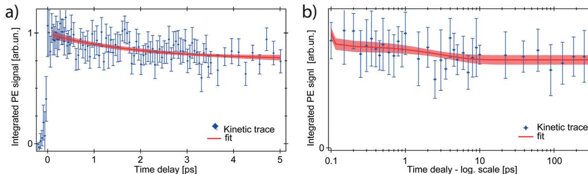
Fig. 5 Kinetic traces of the ferrous PE signal. (a) 5 ps range with LAPE subtracted: a partial intensity drop is observed. The red trace shows the fit with exponentially decreasing component  $A_2$  ( $\tau_2 = 2$  ps). (b) Long-time evolution of the PE signal (up to 250 ps): the ferrous PE signal stabilises to an asymptotic value, which remains for the whole time window.
