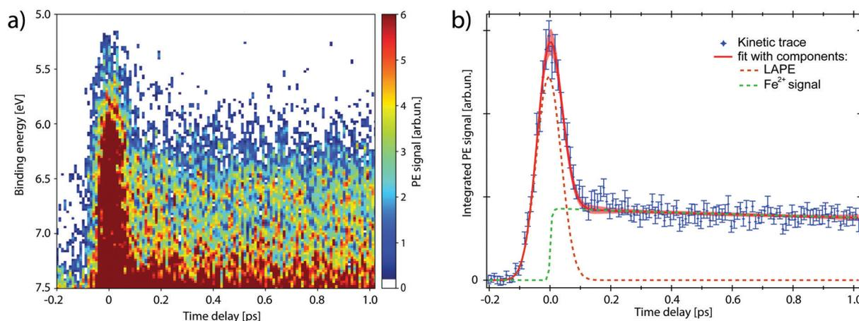
Fig. 4 Time-resolved PE spectra of the ferrioxalate aqueous solution ( $h\nu = 34$  eV) impulsively excited at 263 nm. (a) 2D map in the energy range where the transient signal and LAPE overlap. (b) Kinetic trace of the transient signal (blue). The fit (red) is plotted with its components: LAPE (orange) and transient signal (green), showing a rise-time much faster than the experimental time resolution (see text for details).
