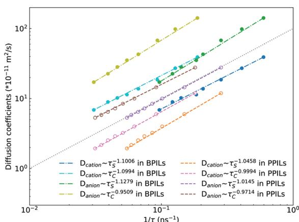
Fig. 22 Diffusion coefficients of PIL cation monomers ( $D_{\text{cation}}$ ) and anions ( $D_{\text{anion}}$ ) against ion pairing association times ( $\tau_S$ ) and ion structural relaxation times ( $\tau_C$ ). The dotted grey line with a slope of 1 represents a guide to the eye.
