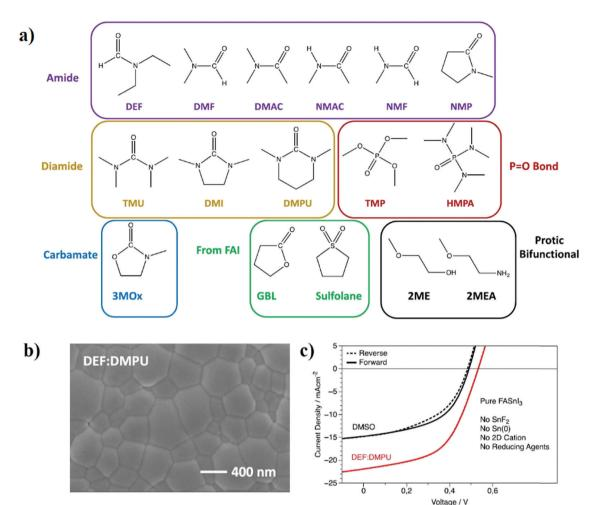
Fig. 4 (a) 16 nonsulfoxide solvents that formed stable perovskite solution divided into groups according to the functional group. (b) SEM images of the DEF:DMPU film. (c) J-V curves of FASnl<sub>3</sub> without any additives in DEF:DMPU against DMSO.<sup>78</sup> Reproduced with permission Copyright 2021, American Chemical Society
