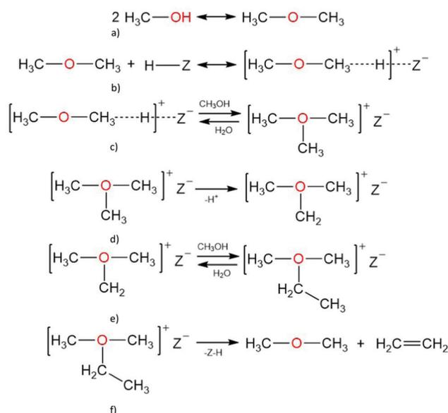
**Scheme 1** Ethene formation *via* the oxonium ylide mechanism, starting from (a) methanol and (b) dimethyl ether, followed by (c) dimethyl ether activation to form (d) trimethyl oxonium, which is (e) deprotonated and (f) converted to dimethyl ethyl ether resulting in (g) ethene and dimethyl ether.
