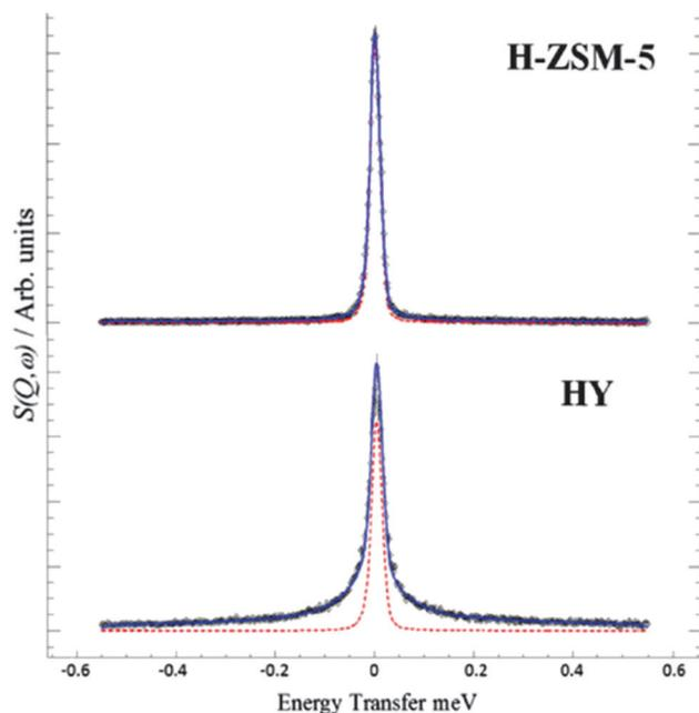
Fig. 10 QENS spectra at 298 K of methanol loaded in zeolites H-ZSM-5 and HY at  $Q = 0.9 \text{ \AA}^{-1}$ , (--) represents the resolution data taken at 5 K. Reprinted from ref. 172 with permission of the Royal Society of Chemistry.
