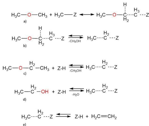
**Scheme 4** Ethene formation *via* the methoxymethyl/ethoxy mechanism, where (a) dimethyl ether polarises methoxy, which leads to (b) the production of methanol and ethoxy; (c) ethyl methyl ether and (d) ethanol convert to zeolite bound ethoxy that (e) produces ethene.
