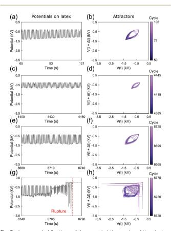
Fig. 3 (a, c, e and g) Sections of the recorded time series of the electrostatic potential of the periodically stretched natural latex and (b, d, f and h) the respective attractors. See also Fig. S3 and S5 (ESI†).
