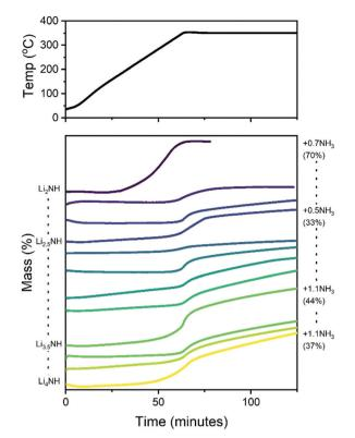
Fig. 8 Simultaneous thermal analysis data for lithium imide-nitridehydride samples heated under a constant flow of ammonia. Indicated on the right are the upper bounds of absorbed molar equivalents of ammonia by selected samples (assuming all mass gain is through ammonia absorption), along with the extent of reaction towards lithium amide
