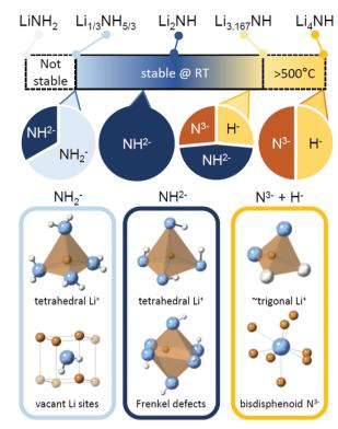
Fig. 7 A summary of the stable composition range of the Li-N-H solid solution, along with key structural features expected for samples dominate by amide, imide or nitride-hydride anions.
