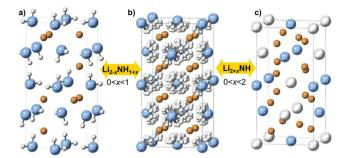
Fig. 1 Crystal structures of (a) lithium amide (b) lithium imide with disordered hydrogen positions (>80 °C) and (c) lithium nitride-hydride, with solid solutions indicated in between structures. Lithium is shown in orange, nitrogen in blue, and hydrogen in white
