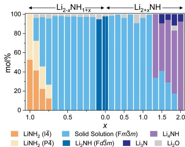
Fig. 3 Phase composition as determined by Rietveld analysis of synchrotron powder X-ray diffraction data.
