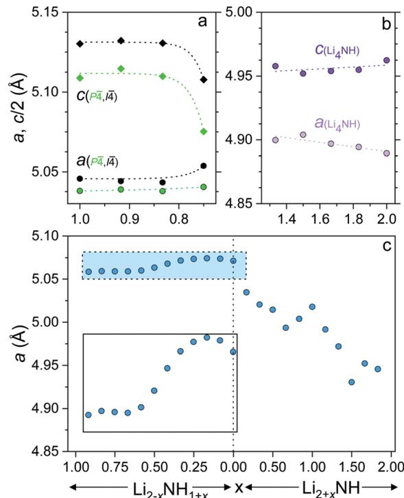
**Fig. 4** Lattice parameters of (a) lithium amide (b) lithium nitride–hydride and (c)  $Fm\bar{3}m$  phases (and  $0.5 \times a$  for the  $Fd\bar{3}m$   $\text{Li}_2\text{NH}$  phase), with an inset plot of the highlighted amide–imide region. Error bars are smaller than the data points.
