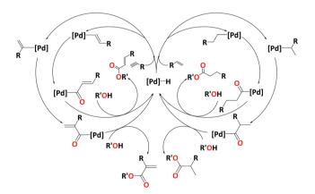
Scheme 2 Catalytic cycles for alkoxycarbonylation of alkynes (left) and alkenes (right) emerging from a [Pd]-H complex, showing the formation of branched (outer cycle) and linear products (inner cycle).
