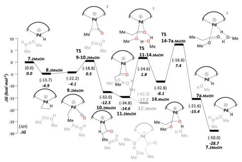
Scheme 5 Hydride-hydroxyalkylpalladium pathway (pathway C in the original paper): free energy profile using methanol as the model solvent at the B3PW91-D3/6-311G\*\*/SDD/PCM level. Energies are in kcal mol<sup>-1</sup> relative to 7•2MeOH. Explicit solvent molecules are shown in light grey colour. The ligand DTBPX, is shown in Scheme 1(i). Reprinted from ref. 98 (Copyright 2020 Royal Society of Chemistry).
