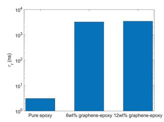
Fig. 5 Rotational relaxation time of bisphenol F molecules in pure epoxy and graphene-bound bisphenol F molecules in GFI epoxy systems.
