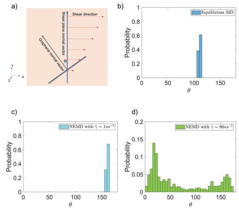
Fig. 7 Probability distribution of the angle [shown schematically in (a)] between the graphene normal vector and the y-axis (normal vector to the shear planes in NEMD simulations) in the (b) absence and (c and d) presence of shear flow for the case of 6 wt% graphene infused epoxy system.
