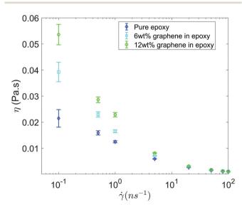
Fig. 3 Viscosity as a function shear rate for all the three systems considered in this study. Error bars are estimated using the block averaging method. Block sizes are chosen as the value beyond which the standard error plateaus out.
