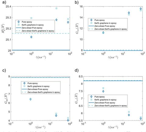
Fig. 6 (a) Mean-squared radius of gyration, (b)  $G_{xx}$  (c)  $G_{yy}$  and (d)  $G_{zz}$  of bisphenol F molecules, in pure epoxy and GFI epoxy, in the presence and in the absence of shear slow
