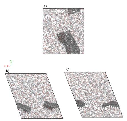
Fig. 2 Simulation snapshots of 6 wt% graphene infused epoxy ink (a) in the absence of shear rate (EMD) and in the presence of a shear rate (NEMD) of (b) 1 ns<sup>-1</sup> and (c) 80 ns<sup>-1</sup>.
