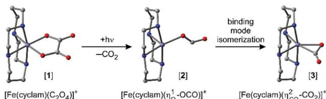
**Fig. 1** Molecular structures of the ferric oxalato-iron(III) parent complex, **[1]**, the primary ferrous product, **[2]**, exhibiting an O-“end-on” bound carbon dioxide radical anion ligand, and the secondary (ferroxycyclopropane) product, **[3]**, featuring a “side-on” bound  $\text{CO}_2$ -ligand (see text for details).
