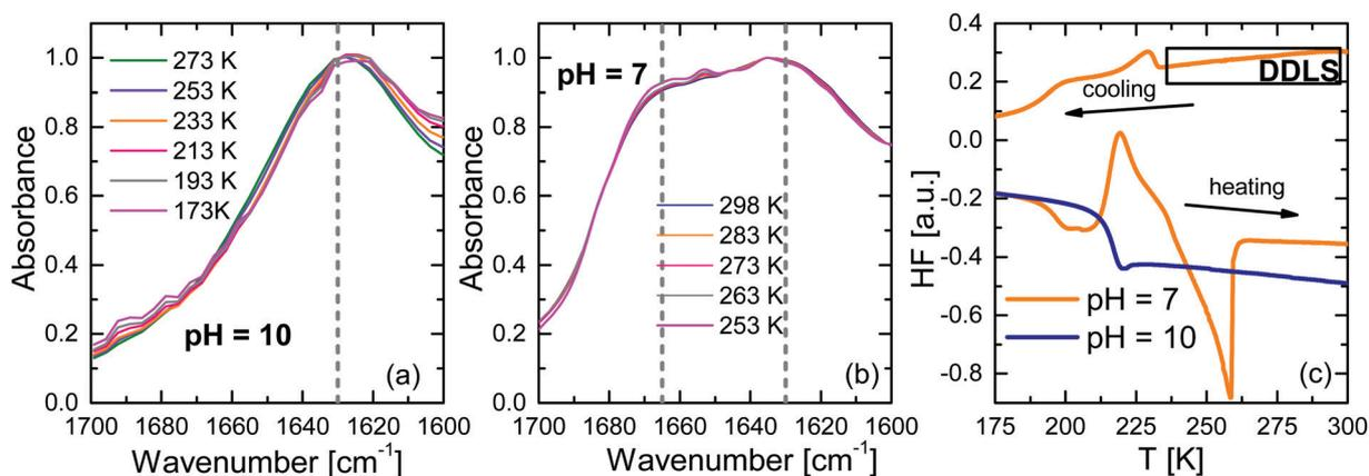
Fig. 1 (a) Amide I band (1630 cm<sup>-1</sup>) of the infrared spectra of  $\epsilon$ -PLL, pH = 10 sample and amide I bands (1630 and 1665 cm<sup>-1</sup>) for pH = 7 sample at different temperatures indicated in the figure. (c) DSC scans measured at 5 K min<sup>-1</sup> for both pH values; for the pH = 7 sample, the temperature range over which the DDLS measurements were made is shown.
