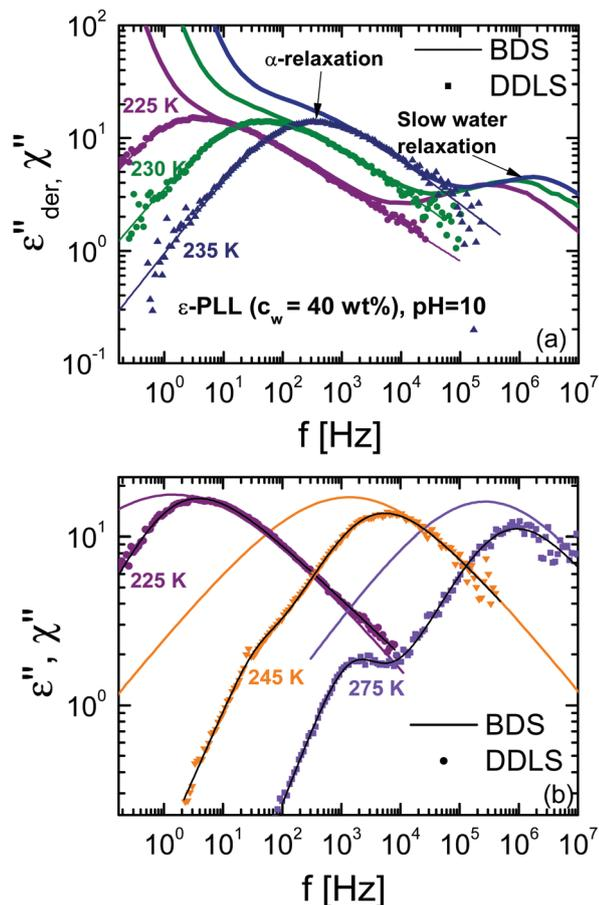
Fig. 8 (a) Comparison of dielectric data (lines) and DDLs data (symbols) at different temperatures for  $\epsilon$ -PLL, pH = 10. In (b) we compare the  $\alpha$ -relaxation obtained from the fitting of the dielectric data with the susceptibilities at different temperatures as indicated in the figure.
