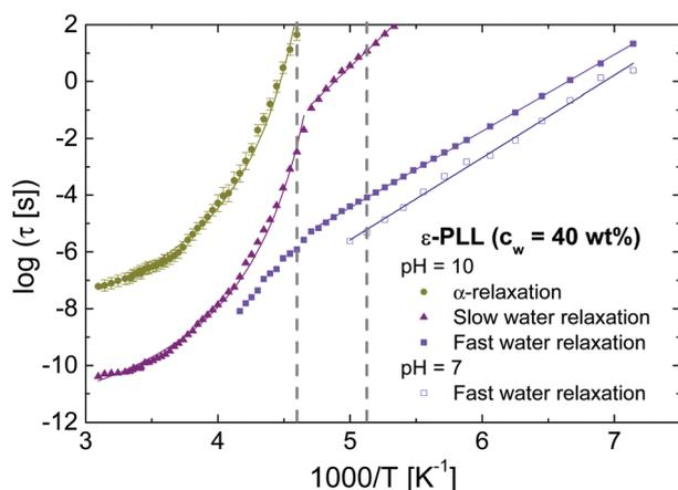
Fig. 3 Temperature dependence of the relaxation times of  $\epsilon$ -PLL solutions obtained from BDS at two pH values. The vertical dashed lines indicate the glass transition temperature  $T_g = 217$  K for pH = 10 and 195 K for pH = 7.
