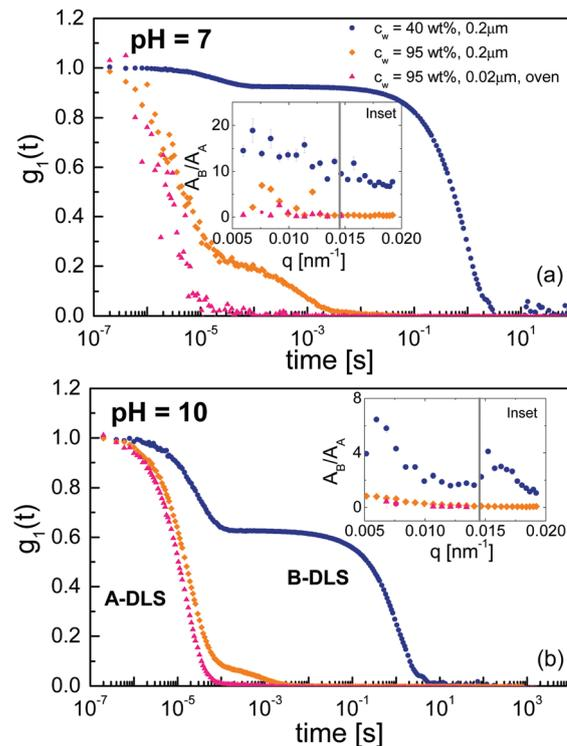
Fig. 6 Normalized PDS electric field correlation function ( $g_1(t)$ ) for  $\epsilon$ -PLL–water solution of (a) pH = 7 and (b) pH = 10 at room temperature and a scattering angle of  $\theta = 90^\circ$ , showing the B-DLS and A-DLS processes. The insets show the ratio of the amplitudes of both processes ( $A_B/A_A$ ) as a function of the  $q$  value.
