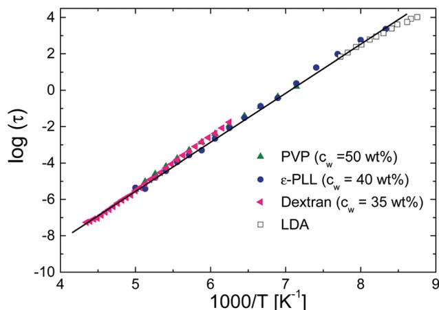
Fig. 11 Temperature dependence of the relaxation times of the fast-water relaxations in different systems ( $\epsilon$ -PLL at pH = 10, low density amorphous ice (LDA),<sup>56</sup> poly(vinyl pyrrolidone)<sup>13</sup> and dextran<sup>14</sup>).
