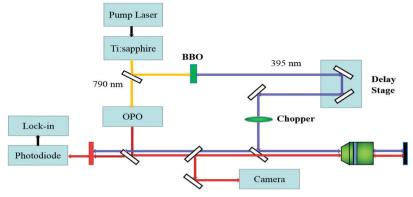
Fig. 2 Schematic of the transient absorption microscope setup.
