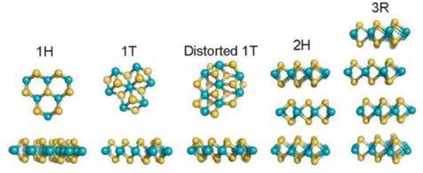
Fig. 4 Crystal structures of MoS<sub>2</sub> with different polymorphisms. Reproduced from ref. 73 with permission from American Chemical Society.
