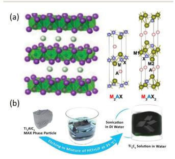
Fig. 7 (a) Atomic and crystal structure MAX phases. Reproduced from ref. 91 with permission from American Chemical Society. (b) Schematic of the Ti<sub>3</sub>C<sub>2</sub>T<sub>x</sub> synthesis procedure. Reproduced from ref. 93 with permission from American Chemical Society
