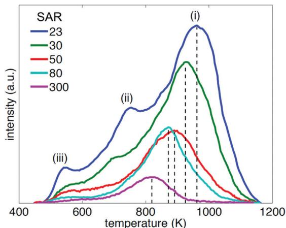
Fig. 3 Mass-normalised TPD spectra of pyridine in HZSM-5 with varying silica/alumina ratios (SAR) acquired with a heating rate of  $10 \text{ K min}^{-1}$ . Dashed lines indicate the position of the maximum desorption rate for each material.
