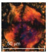
Fig. 3 POM texture of compound 4a in (left) the nematic phase at 136 °C and (right) the twist-bend nematic phase at 96 °C.
