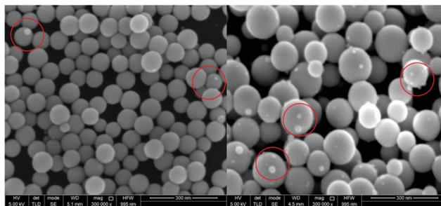
Fig. 10 SEM images of gallium deposits generated from DME containing  $0.1 \text{ mol dm}^{-3}$  of  $\text{GaCl}_3$  and  $0.2 \text{ mol dm}^{-3}$  of  $[\text{TBA}][\text{ClO}_4]$  by applying  $-1.5 \text{ V vs. Fc}^+/\text{Fc}$  for 1 min on a GC WE at  $26^\circ \text{C}$ . The applied acceleration voltage was 5 keV.
