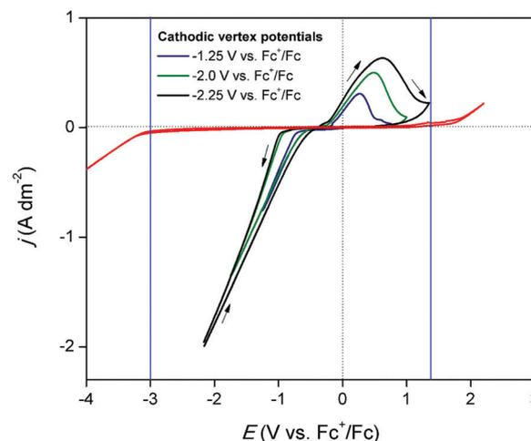
Fig. 2 CVs recorded on a GC WE ( $\varnothing = 4$  mm) for DME containing 0.1 mol dm<sup>-3</sup> of GaCl<sub>3</sub> and 0.2 mol dm<sup>-3</sup> of [TBA][ClO<sub>4</sub>] (black), scanned to different vertex potentials at a scan rate of 20 mV s<sup>-1</sup> at 26 °C.
