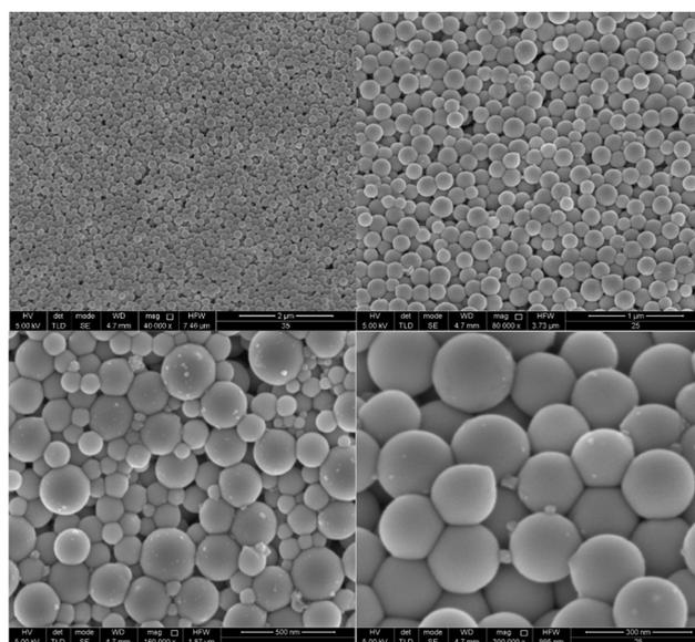
Fig. 6 SEM images of gallium deposits generated from DME containing 0.1 mol dm<sup>-3</sup> of GaCl<sub>3</sub> and 0.2 mol dm<sup>-3</sup> of [TBA][ClO<sub>4</sub>] by applying -1.5 V vs. Fc<sup>+</sup>/Fc for 30 min. on a GC WE at 26 °C. The applied acceleration voltage was 5 keV.
