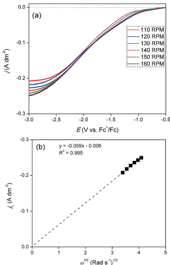
Fig. 5 (a) LSVs recorded on a GC disk electrode ( $\varnothing = 5$  mm) for DME containing 10 mmol dm<sup>-3</sup> of GaCl<sub>3</sub> and 0.2 mol dm<sup>-3</sup> of [TBA][ClO<sub>4</sub>] at various rotation rates, at a scan rate of 10 mV s<sup>-1</sup>, at 26 °C. (b) Levich plot constructed using the limiting current densities of the LSVs at -3.0 V vs. Fc<sup>+</sup>/Fc.
