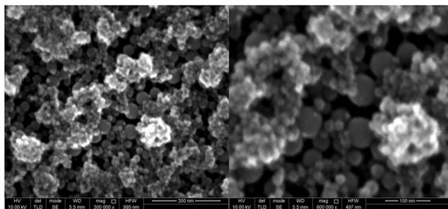
Fig. 11 SEM images of gallium structures generated by first electrodepositing gallium from DME containing  $0.1 \text{ mol dm}^{-3}$  of  $\text{GaCl}_3$  and  $0.2 \text{ mol dm}^{-3}$  of  $[\text{TBA}][\text{ClO}_4]$  by applying  $-1.5 \text{ V}$  vs.  $\text{Fc}^+/\text{Fc}$  for 2 min and then partly stripping the deposited gallium by applying  $+0.2 \text{ V}$  vs.  $\text{Fc}^+/\text{Fc}$  for 1 min at  $26^\circ\text{C}$ . The applied acceleration voltage was 10 keV.
