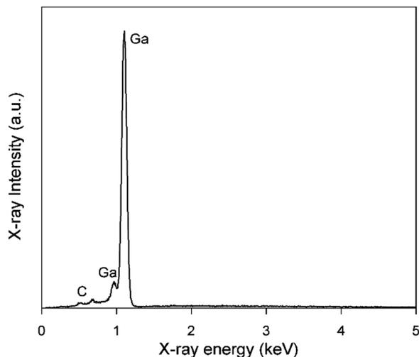
Fig. 7 EDX spectrum of gallium deposits generated from DME containing  $0.1 \text{ mol dm}^{-3}$  of  $\text{GaCl}_3$  and  $0.2 \text{ mol dm}^{-3}$  of  $[\text{TBA}][\text{ClO}_4]$  by applying  $-1.5 \text{ V}$  vs.  $\text{Fc}^+/\text{Fc}$  for 30 min on a GC WE at  $26^\circ\text{C}$ . The applied acceleration voltage was 10 keV.
