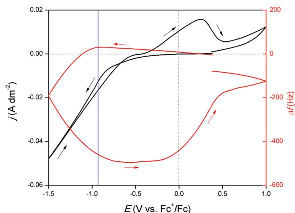
Fig. 3 CV recorded on a 5 MHz platinum-coated quartz crystal ( $\varnothing = 12.4$  mm) for DME containing  $10 \text{ mmol dm}^{-3}$  of  $\text{GaCl}_3$  and  $0.1 \text{ mol dm}^{-3}$  of  $[\text{TBA}][\text{ClO}_4]$  at a scan rate of  $10 \text{ mV s}^{-1}$  at  $26^\circ\text{C}$  (full line left axis) with EQCM analysis (right axis).
