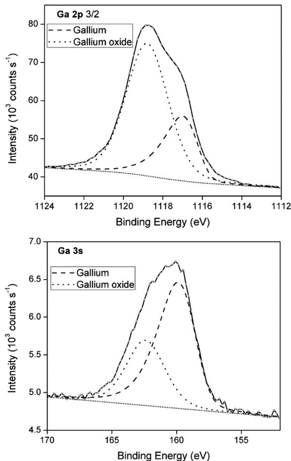
Fig. 8 Curve-fitted Ga 2p<sub>3/2</sub> and Ga 3s XPS spectra from deposits generated from DME containing  $0.1 \text{ mol dm}^{-3}$  of  $\text{GaCl}_3$  and  $0.2 \text{ mol dm}^{-3}$  of  $[\text{TBA}][\text{ClO}_4]$  by applying  $-1.5 \text{ V}$  vs.  $\text{Fc}^+/\text{Fc}$  for 30 min on a GC WE at  $26^\circ\text{C}$ .
