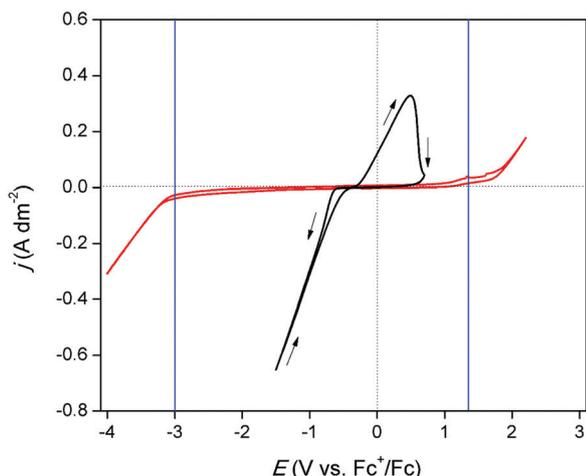
Fig. 1 CVs recorded on a GC WE ( $\varnothing = 4$  mm) for DME containing 0.2 mol dm<sup>-3</sup> of [TBA][ClO<sub>4</sub>] (red) and DME containing 0.1 mol dm<sup>-3</sup> of GaCl<sub>3</sub> and 0.2 mol dm<sup>-3</sup> of [TBA][ClO<sub>4</sub>] (black) at a scan rate of 20 mV s<sup>-1</sup> at 26 °C.
