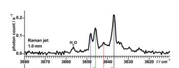
Fig. 10 Raman jet spectrum of 2-methyl-2-butanol in comparison with a simulation. For the latter the PBE0-D3 harmonic wavenumbers are corrected as proposed by our model and a Lorentzian broadening of FWHM =  $1.5 \text{ cm}^{-1}$  is applied. A Boltzmann distribution at 100 K is assumed.
