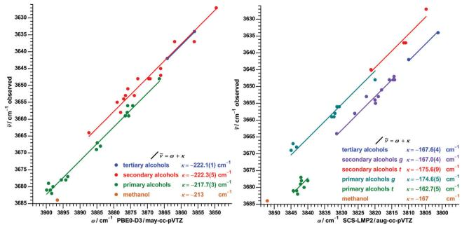
Fig. 3 Correlation between observed OH stretch fundamental wavenumbers  $\tilde{\nu}$  and calculated harmonic wavenumbers  $\omega$  for alcohols at PBE0-D3 (left) and SCS-LMP2 (right) level. Separate for selected alcohol classes a linear regression  $\tilde{\nu} = \omega + \kappa$  was performed with a fixed slope of unity and an optimized intercept  $\kappa$  with standard error in parentheses.
