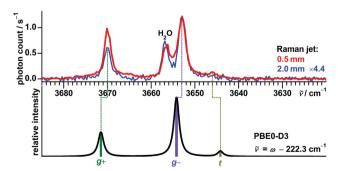
Fig. 8 Raman jet spectra of (–)-borneol at two detection distances from the nozzle scaled to similar intensities of the 3653  ${\rm cm}^{-1}\,{\rm signal},$  in comparison with a simulated spectrum. For the simulation the PBE0-D3 harmonic wavenumbers are corrected as proposed by our model and a Lorentzian broadening of FWHM = 1.5 cm<sup>-1</sup> is applied. A Boltzmann distribution at 100 K is assumed.
