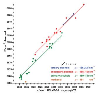
Fig. 2 Correlation between observed OH stretch fundamental wavenumbers  $\tilde{\nu}$  and calculated harmonic wavenumbers  $\omega$  for alcohols at B3LYP-D3 level. Separate for each alcohol class a linear regression  $\tilde{\nu} = \omega + \kappa$  was performed with a fixed slope of unity and an optimized intercept  $\kappa$  with standard error in parentheses.
