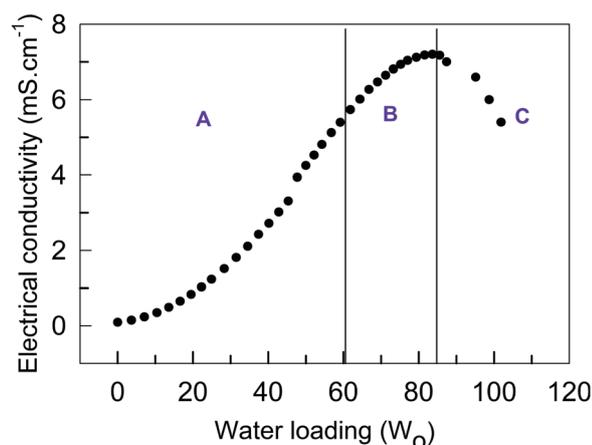
Fig. 7 Electrical conductivity ( $\text{mS cm}^{-1}$ ) as a function of water loading ( $w_o$ ) in water/TX-100 (300 mM)/TBAC-DA microemulsion at ambient conditions. Regions A, B, and C are described in the text.
