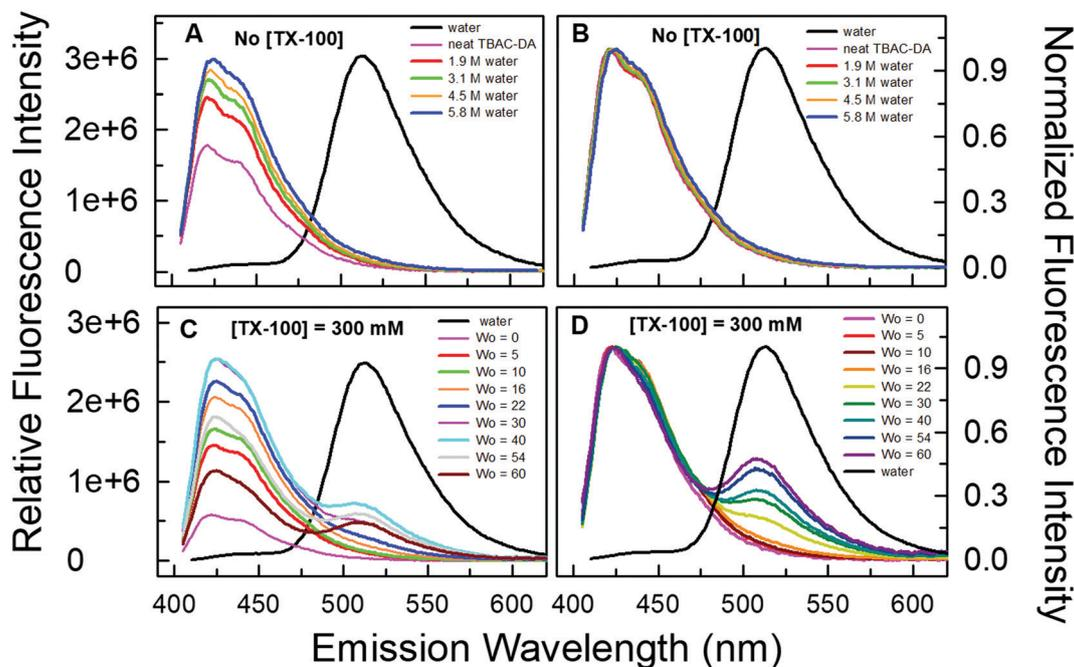
Fig. 4 Relative (panels A and C) and normalized (panels B and D) fluorescence emission spectra of pyranine (10  $\mu\text{M}$ ,  $\lambda_{\text{ex}} = 390$  nm, and slits: excitation/emission = 2/2 nm) dissolved within neat DES TBAC-DA and TX-100(300 mM)/TBAC-DA systems at different amounts of water loading ( $w_0$ ), respectively. The fluorescence emission spectrum of pyranine in water is also included in each panel for reference.
