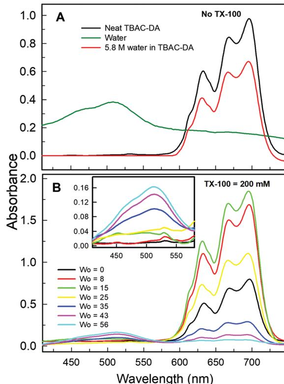
Fig. 5 UV-vis absorbance spectra of  $\text{Co}^{\text{II}}$  within water, neat TBAC-DA, and water saturated TBAC-DA (panel A) and the TX-100 (200 mM)/TBAC-DA system (panel B) at different amounts of water loading ( $w_0$ ). Inset in panel B is the magnified portion of the plot for clear depiction of the peak at  $\sim 509$  nm.
