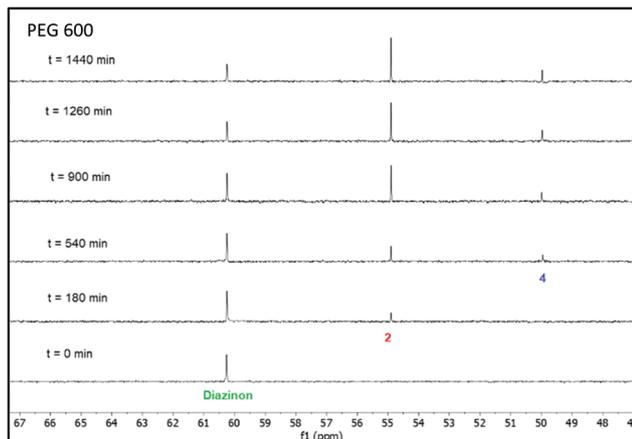
Fig. 5 Stacked  $^{31}\text{P}$ -NMR spectra for the nucleophilic degradation of diazinon with piperidine performed in a mixture of 35 wt% PPG 400 + 15 wt% PEG 600 + 50 wt%  $\text{H}_2\text{O}$  at 298 K.
