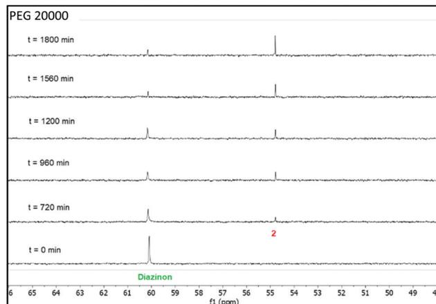
Fig. 7 Stacked  $^{31}\text{P}$ -NMR spectra for the nucleophilic degradation of diazinon with piperidine performed in a mixture of 35 wt% PPG 400 + 15 wt% PEG 20 000 + 50 wt%  $\text{H}_2\text{O}$  at 298 K.
