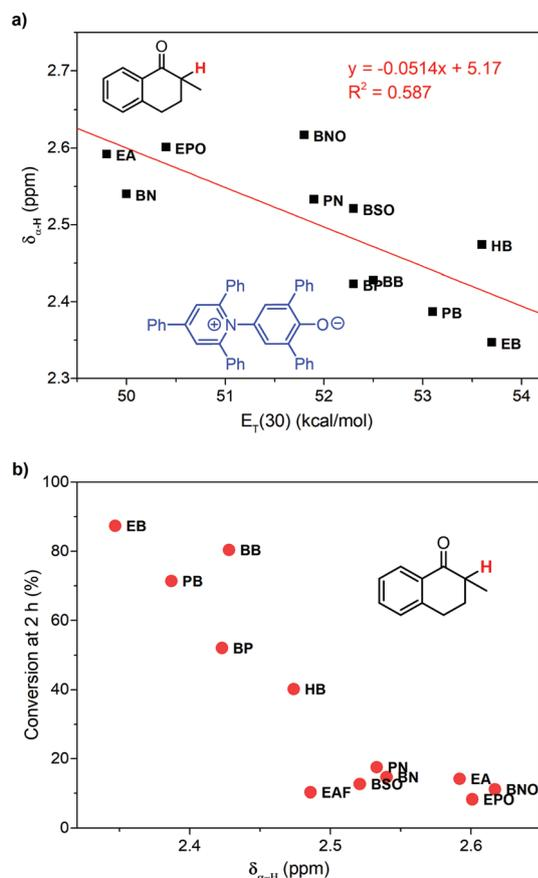
Fig. 4 (a) Correlated chemical shift of the  $\alpha$ -proton in **1** with the  $E_T(30)$  value in 1-alkyl-3-methylimidazolium ILs. (b) The relationship between the conversion of **1** at 2 h and the chemical shift of the  $\alpha$ -proton in **1**.
