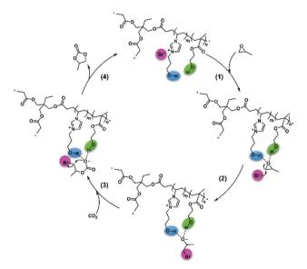
Scheme 4  $\,$  Proposed possible mechanism for  $CO_2$  cycloaddition with PO catalyzed by HPIL-7.
