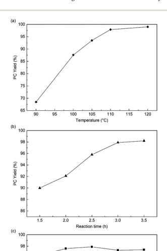
Fig. 4 The effects of different reaction conditions to PC yield. Reaction conditions: PO (0.83 g, 14.3 mmol), HPIL-7 (180 mg, 1.5 mol%, based on the EA results), (a) 2 MPa  $\rm CO_2$ , 3 h. (b) 110 °C, 1.5 MPa (c) 110 °C, 3 h.
