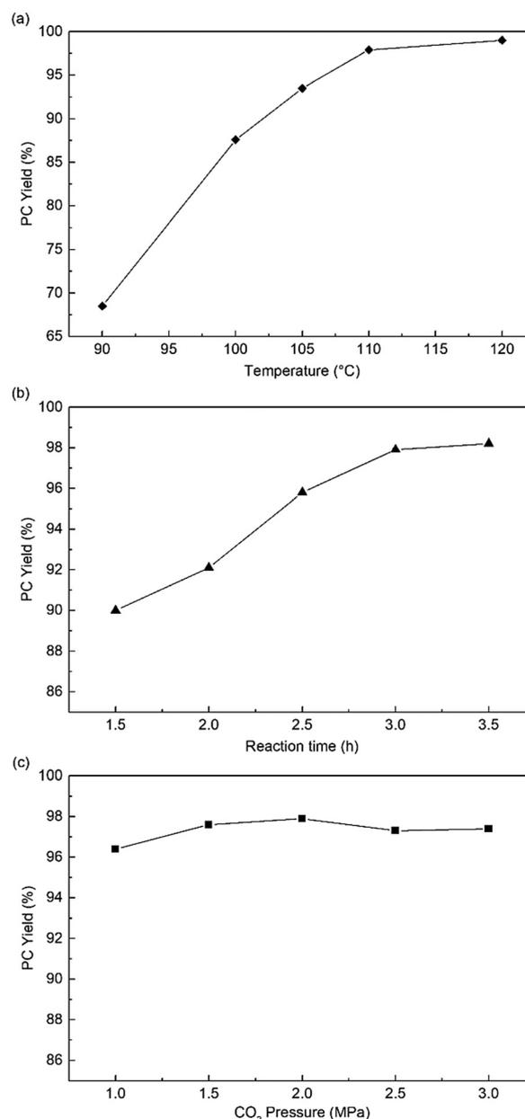
Fig. 4 The effects of different reaction conditions to PC yield. Reaction conditions: PO (0.83 g, 14.3 mmol), HPIL-7 (180 mg, 1.5 mol%, based on the EA results), (a) 2 MPa CO<sub>2</sub>, 3 h. (b) 110 °C, 1.5 MPa (c) 110 °C, 3 h.
