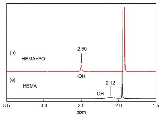
Fig. 8  $^1\text{H}$  NMR spectra of HEMA with and without PO in  $\text{CDCl}_3$ . (a) HEMA 10  $\mu\text{L}$ ,  $\text{CDCl}_3$  0.5 mL. (b) PO 30  $\mu\text{L}$ , HEMA 10  $\mu\text{L}$ ,  $\text{CDCl}_3$  0.5 mL.
