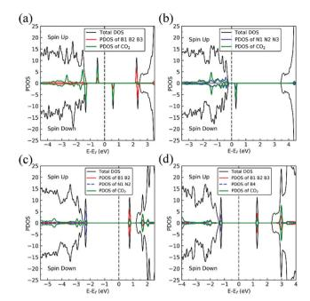
Fig. 14 Spin-polarized total density of states (TDOS) (black line), and spin-polarized PDOS of defect area (red line or blue line) and of adsorbed CO<sub>2</sub> (green line) of CO<sub>2</sub>–dh-BN with (a)  $V_{\rm N}$ , (b)  $V_{\rm B}$ , (c) SW, and (d)  $B_{\rm N}$ , respectively. The position of the Fermi level ( $E_{\rm F}$ ) is indicated by dashed line.
