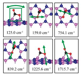
Fig. 17 Notable vibrational modes of  ${\rm CO_2}$  adsorption on dh-BN with SW. The magenta, blue, black and red balls represent the B, N, C, and O atoms, respectively. Arrows indicate vibrational patterns. The square in 124.6 cm $^{-1}$  mode figure (left) encloses all atoms that concertedly vibrate together.
