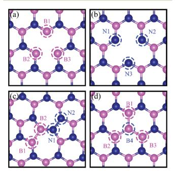
Fig. 1 Schematic representation of h-BN model systems with defects: (a)  $V_N$ , (b)  $V_B$ , (c) SW, and (d)  $B_N$ . Blue and magenta balls represent N and B
