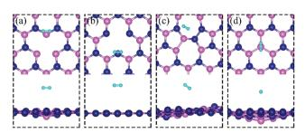
Fig. 3 Optimized structures of  $H_2$  adsorbed at favored sites of h-BN with (a)  $\rm V_{N},$  (b)  $\rm V_{B},$  (c) SW, and (d)  $\rm B_{N}.$  The magenta, blue, white balls represent the B, N and H atoms, respectively. The top and bottom panel shows the top and side views, respectively.
