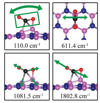
Fig. 18 Notable vibrational modes of  $CO_2$  adsorption on dh-BN with  $B_N$ . The magenta, blue, black and red balls represent the B, N, C, and O atoms, respectively. Arrows indicate vibrational patterns. The rectangular in the left figure encloses atoms that concertedly vibrate together.
