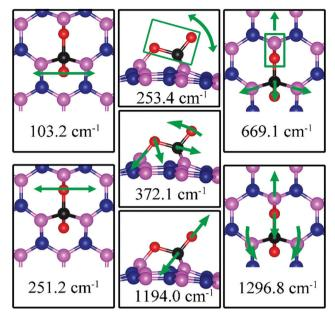
Fig. 15 Notable vibrational modes of CO<sub>2</sub> adsorption on dh-BN with V<sub>N</sub>. The magenta, blue, black and red balls represent the B, N, C, and O atoms, respectively. Arrows indicate vibrational patterns. The rectangular encloses the atoms that move together.
