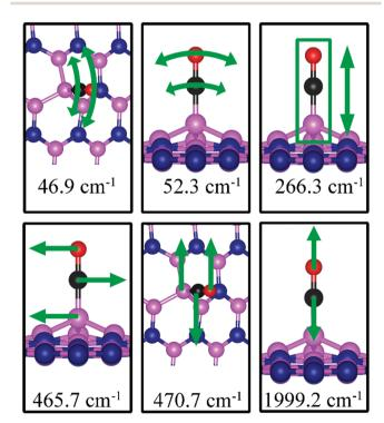
Fig. 12 Notable vibrational modes of CO adsorption on dh-BN with B<sub>N</sub>. The magenta, blue, black and red balls represent the B, N, C, and O atoms, respectively. Arrows indicate vibrational patterns. The rectangular encloses the atoms that are concertedly move together.
