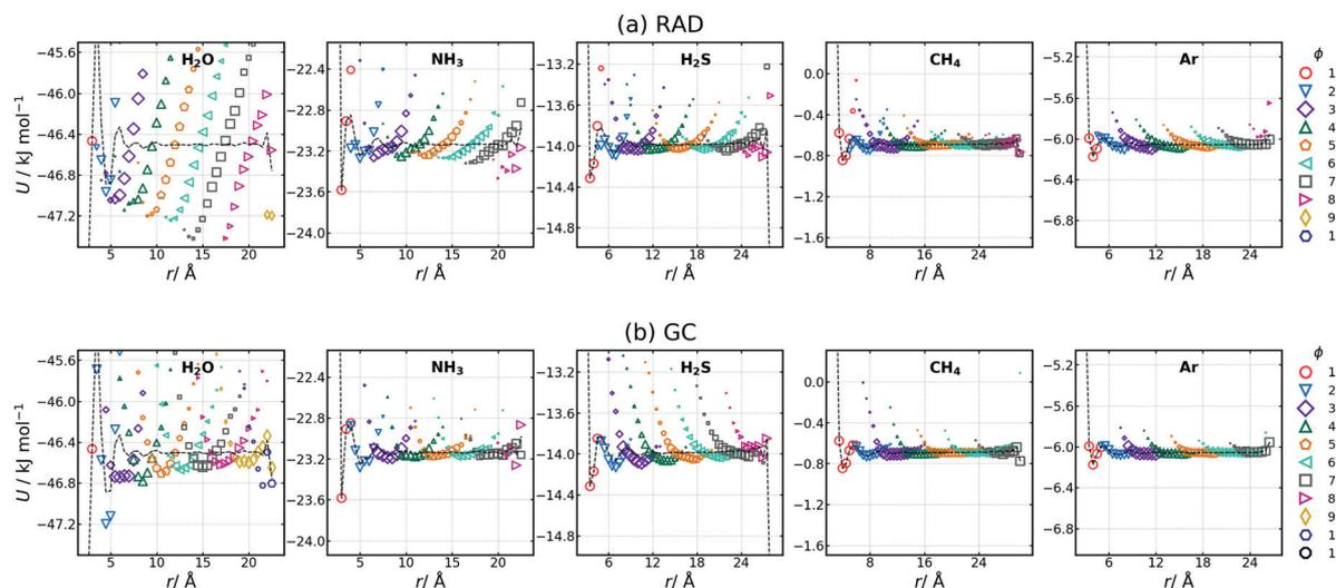
Fig. 3 Potential energy  $U$  of a molecule in a particular shell  $\phi$  and distance  $r$  from the reference molecule for shells defined by (a) RAD or (b) GC. Averaged energy by distance is shown with a black dashed-line. Each marker represents an  $r$  bin value of  $0.5 \text{ \AA}$  that is colored and shaped according to the shell index and sized according to its population.
