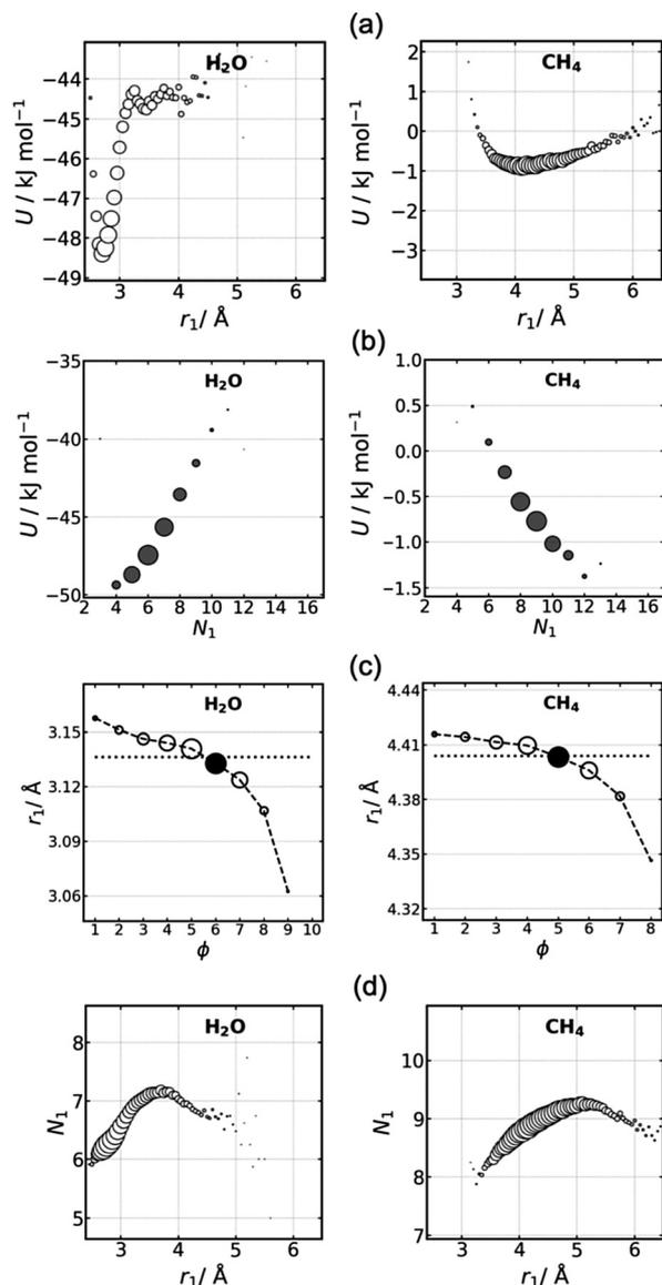
Fig. 4 Effect of (a) coordination radius and (b) number  $N_1$  on potential energy  $U$ , (c)  $r_1$  versus  $\phi$ , and (d)  $N_1$  versus  $r_1$  for water (column 1) and methane (column 2) RAD shells. Marker size represents the population of molecules at each value.
