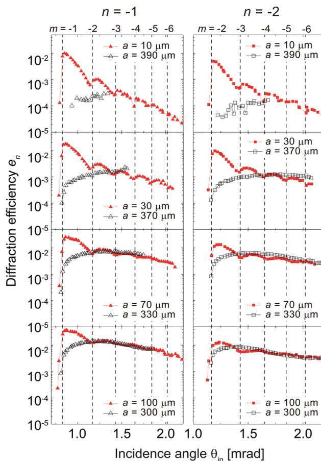
Fig. 5 Diffraction efficiencies of the  $-1$ st-order (left column) and  $-2$ nd-order (right column) plotted as a function of incidence angle  $\theta_{in}$ . The dashed vertical lines indicate Rayleigh angles of emergence of another diffraction beam of order  $m$  as labeled on top of the graphs.
