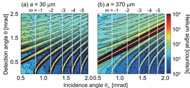
Fig. 3 Contour plots composed of diffraction patterns measured at various incidence angles with two complementary gratings of (a)  $a = 30$   $\mu\text{m}$  and (b) 370  $\mu\text{m}$ . The vertical dashed white lines indicate the Rayleigh incidence angle  $\theta_{R,m}$  where the  $m$ th-order diffraction beam emerges from the grating.<sup>36</sup> The continuous grey lines present the calculated diffraction angles.
