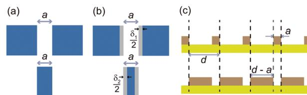
**Fig. 1** (a) A slit and a strip of an identical physical width  $a$ . (b) A slit and a strip of an identical effective width  $a$ . The geometrical width of the slit and the strip are  $a + \delta_1$  and  $a - \delta_2$ , respectively. The difference between the real and the effective widths are illustrated by gray areas. (c) Two square wave gratings of complementary geometries. The period  $d$  is the same for both gratings, while their strip widths are  $a$  and  $d - a$ , respectively.
