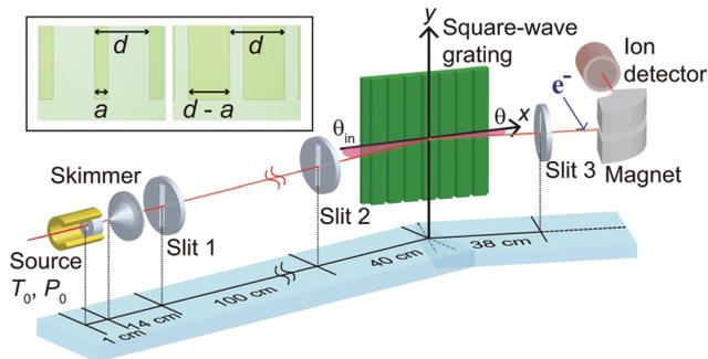
Fig. 2 Schematic of the experimental set-up. The inset shows microscope images of a pair of complementary 400  $\mu\text{m}$ -period gratings with strip widths of 100  $\mu\text{m}$  (left) and 300  $\mu\text{m}$  (right).
