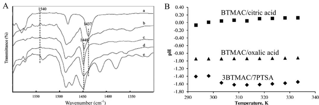
Fig. 7 (A) FT-IR spectra of (a) pure pyridine, (b) pyridine + choline chloride/ZnCl<sub>2</sub>, (c) pyridine + choline chloride/2ZnCl<sub>2</sub>, (d) pyridine + choline chloride/3ZnCl<sub>2</sub> and (e) pyridine + benzyltrimethylammonium chloride/2ZnCl<sub>2</sub>. Reprinted with permission from ref. 60. (B) The dependence of pH on the temperature for three DESs. Reprinted with permission from ref. 62.
