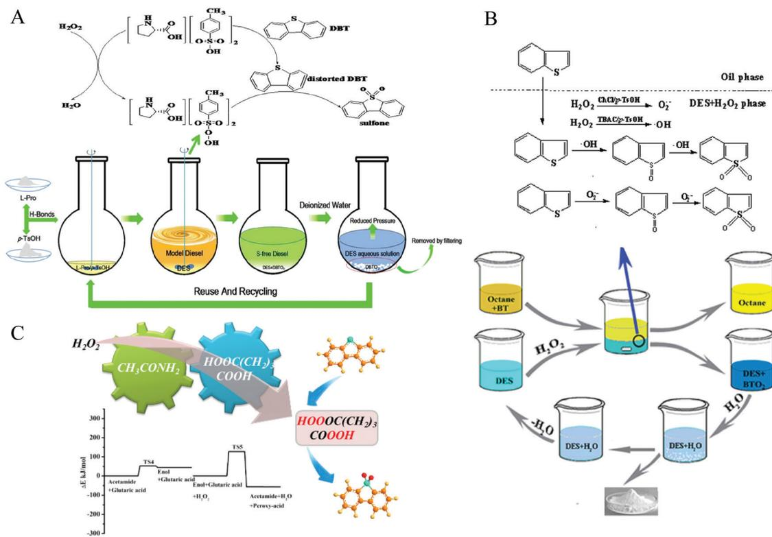
Fig. 9 The mechanism of extraction-oxidation desulfurization using DESs with  $H_2O_2$  as an oxidant. (A) L-Proline/*p*-TsOH DES system. Reprinted with permission from ref. 102. (B) ChCl/*p*-TsOH DES system. Reproduced from ref. 104 with permission from the Royal Society of Chemistry. (C) The reaction potential energy of the oxidation of glutaric acid with the assistance of acetamide. Reprinted with permission from ref. 39.
