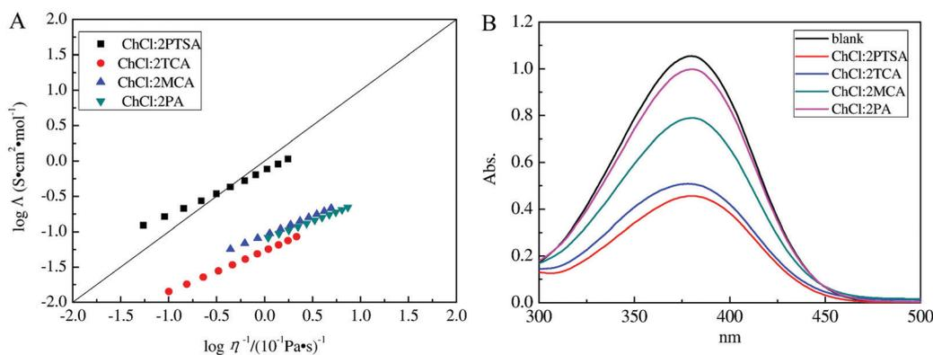
Fig. 6 (A) The dependence of  $\log \Lambda$  on  $\log \eta^{-1}$  for various DESs. The solid straight line is the ideal line for aqueous KCl solutions. (B) UV-vis absorbance spectra of 4-nitroaniline for different DESs in water. Reprinted with permission from ref. 45.
