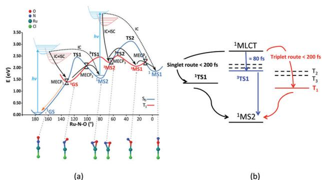
Fig. 7 (a) Mechanism of  $[\text{RuCl}(\text{NO})(\text{py})_4]^{2+}$  photoisomerization based on DFT(B3LYP) and MS-CASPT2 calculations (adapted from ref. 87 with permission from the authors). (b) Three ultrafast decay pathways deduced from TSH dynamics.<sup>67c</sup>
