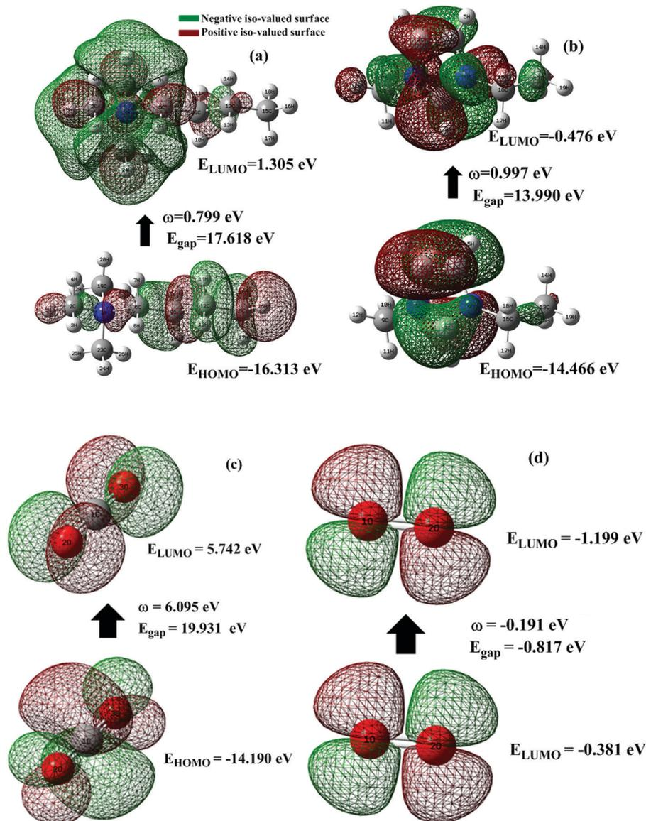
Fig. 2 Frontier molecular orbital showing the 3-D rendered isovalue surface for (a) [BMamm<sup>+</sup>] and (b) [BMIm<sup>+</sup>], (c) CO<sub>2</sub> and (d) O<sub>2</sub><sup>•-</sup>. The green color coding signifies a negative isovalue surface while the brown color coding signifies a positive isovalue surface at the Hartree–Fock/3-21G level of theory.
