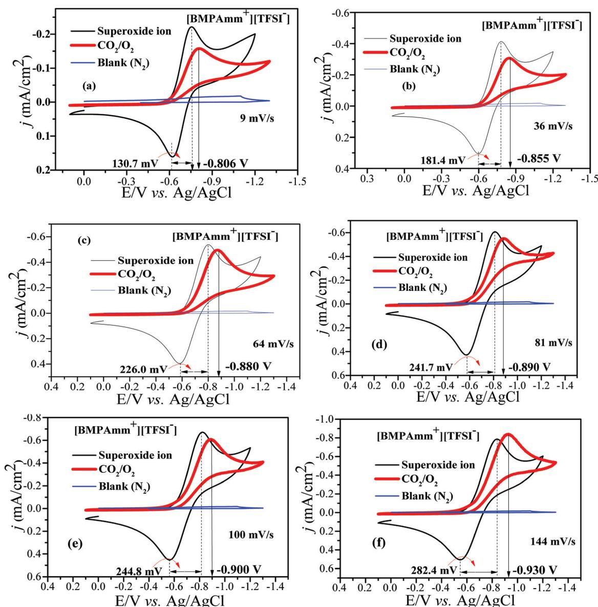
Fig. 5 (a–f) CVs of  $CO_2$  conversion by  $O_2^{\bullet-}$  in [BMAMm<sup>+</sup>][TFSI<sup>-</sup>] after sparging with  $N_2$  (background),  $CO_2$ ,  $O_2$ , and  $CO_2/O_2$  simultaneously at  $27$  °C, GC vs. Ag/AgCl at various sweep rates.
