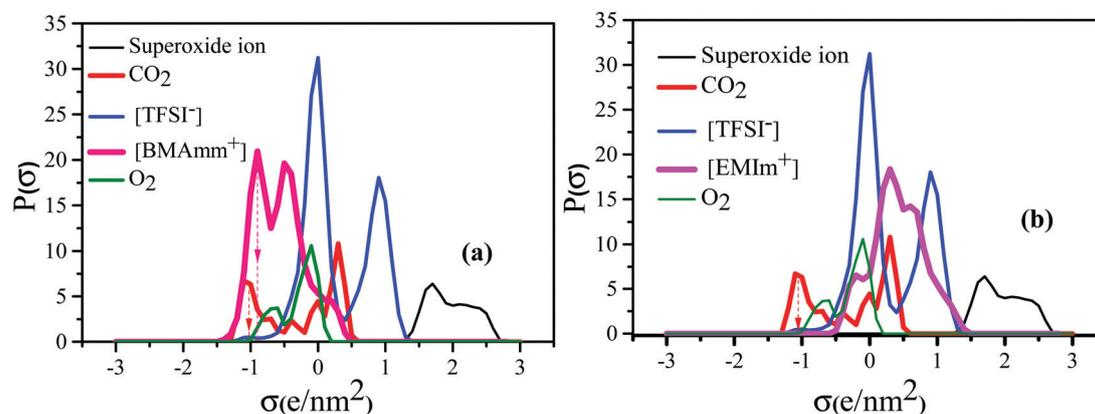
Fig. 1 COSMO RS analysis showing the  $\sigma$ -profile of (a)  $[\text{BMAm}^+]$  and (b)  $[\text{EMIm}^+]$  IL-cations compared with  $[\text{TFSI}^-]$ ,  $\text{O}_2$ ,  $\text{O}_2^{\bullet-}$  and  $\text{CO}_2$ .
