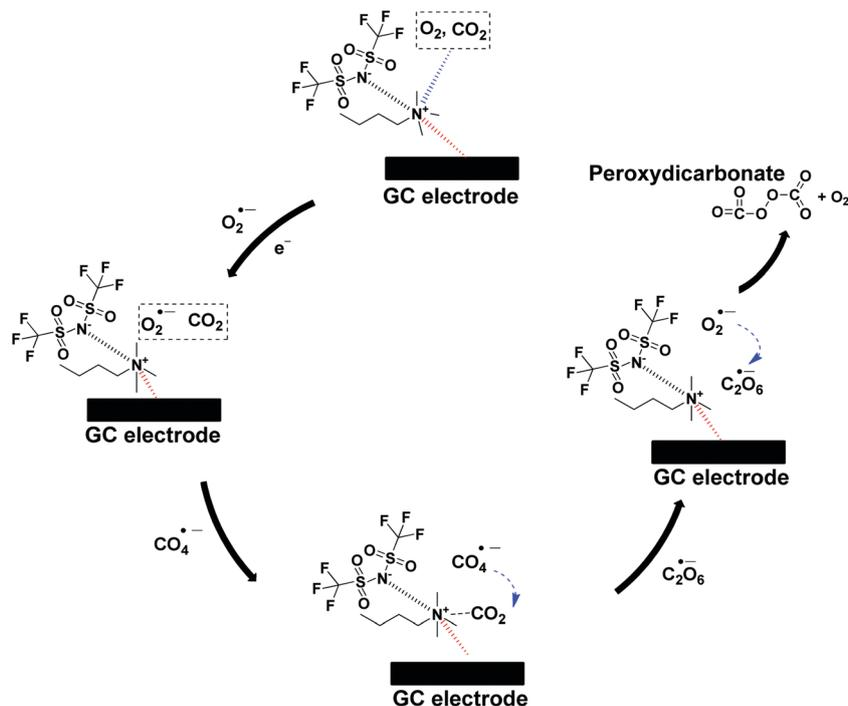
Scheme 2 The proposed mechanism of  $\text{CO}_2$  utilization by  $\text{O}_2^{\bullet-}$  in [BMAm<sup>+</sup>][TFSI<sup>-</sup>].
