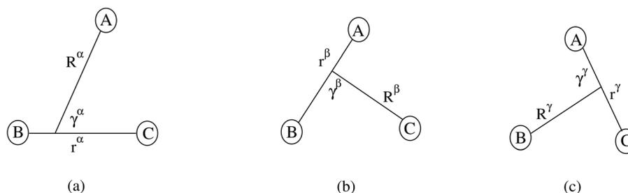
Fig. 1 The Jacobi coordinates for the  $\alpha$ ,  $\beta$  and  $\gamma$  arrangement channels of the A + BC collisional system.
