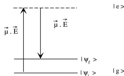
Fig. 2 The ground and the first excited electronic states are represented by  $|g\rangle$  and  $|e\rangle$ , respectively. The wave function for the initial and final vibrational state (for Stokes shift) in the ground electronic state is represented by  $|\psi_i\rangle$  and  $|\psi_f\rangle$ , respectively.
