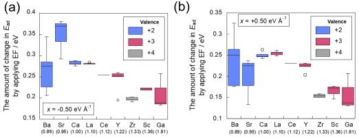
Relationship between the difference of adsorption energy and the electronegativity of the dopant (a) in -0.50 eV Å<sup>-1</sup> and (b) in +0.50 eV Å<sup>-1</sup>.
