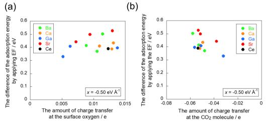
Fig. 8 Relationship between the difference of adsorption energy and the amount of charge transfer: (a) at the surface oxygen and (b) at the CO<sub>2</sub> molecule in -0.50 eV Å<sup>-1</sup>.
