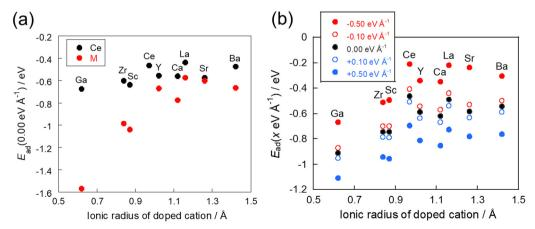
Relationship between the ionic radius and the adsorption energy: (a) without application of an electric field and (b) with application of an electric Fig. 4 field
