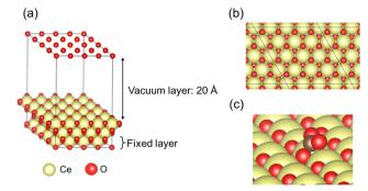
Fig. 1 Calculation models of pure CeO<sub>2</sub>: (a) perspective view, (b) top view, and (c) CO<sub>2</sub> adsorption form on a pure CeO<sub>2</sub>(111) surface: yellow, Ce; red, O
