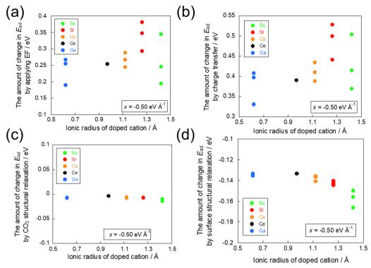
Fig. 7 Effects of factors on the change in the  $CO_2$  adsorption energy in -0.50 eV Å<sup>-1</sup>. The amount of change in the  $CO_2$  adsorption energy (a) by application of EF, (b) by charge transfer, (c) by CO2 molecule structural relaxation, and (d) by surface structural relaxation.
