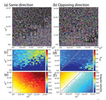
Fig. 3 Dependence of dynamic patterns on the torque strengths  $\omega^{\rm ST}$  and  $\omega^{\text{CT}}$ . (a and b) Time-overlays. (c and d) SPP number fraction within monopolar flocks  $n_{\mathrm{MPF}}$ . To calculate, we first divide the system into 31 imes 31 regions of interest (ROIs), and if an ROI has the polar order parameter
