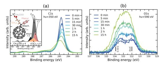
Fig. 1 Experimental (a) C1s XPS spectra and (b) O1s XPS spectra of the unexposed PC<sub>60</sub>BM film and PC<sub>60</sub>BM films exposed to light in air for different durations. The inset of (a) shows the calculated spectrum of pristine PC<sub>60</sub>BM separated into components originating from different molecular moieties, marked with the same colour on the molecular structure. In (b) the binding energies for C-O-C and O=C are indicated, as calculated for pristine PC<sub>60</sub>BM.
