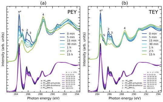
Fig. 9 Experimental C1s NEXAFS in (a) partial electron yield mode, and (b) total electron yield mode of unexposed PC<sub>60</sub>BM and PC<sub>60</sub>BM exposed to light in air for different exposure times (upper part) compared to calculated spectra with different weighted averages between pristine PC<sub>60</sub>BM, PC<sub>58</sub>BManhydride, PC<sub>58</sub>BM-dicarbonyl, and PC<sub>60</sub>BM:O<sub>2</sub> (lower part).
