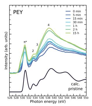
Fig. 3 Measured O1s NEXAFS spectra of unexposed PC<sub>60</sub>BM and PC<sub>60</sub>BM samples exposed to light in air for different durations, shown in comparison to the calculated spectrum of pristine PC<sub>60</sub>BM (black line).
