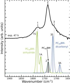
Fig. 6 Measured IR spectrum in the carbonyl region of PC<sub>60</sub>BM exposed to light in air for 47 h (black line, upper part), shown in comparison to the calculated IR spectrum (lower part) of pristine PC<sub>60</sub>BM (black line, shaded grey), PC<sub>58</sub>BM-anhydride (green line) and PC<sub>58</sub>BM-dicarbonyl (blue line). These spectra have been broadened using Gaussian functions of 10 cm<sup>-1</sup> FWHM. The bar graphs represent the calculated IR peak positions and intensities.
