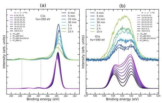
Fig. 8 Experimental (a) C1s XPS and (b) O1s XPS spectra of unexposed  $PC_{60}BM$  and  $PC_{60}BM$  exposed to light in air for different exposure times (upper part) compared to calculated spectra with different weighted averages between pristine PC<sub>60</sub>BM, PC<sub>58</sub>BM-anhydride, PC<sub>58</sub>BM-dicarbonyl, and PC<sub>60</sub>BM:O<sub>2</sub> (lower part):
