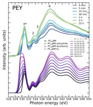
Fig. 10 Experimental O1s NEXAFS of unexposed  $PC_{60}BM$  and  $PC_{60}BM$ exposed to light in air for different exposure times (upper part) compared to calculated spectra with different weighted averages between pristine PC<sub>60</sub>BM, PC<sub>58</sub>BM-anhydride, PC<sub>58</sub>BM-dicarbonyl, and PC<sub>60</sub>BM:O<sub>2</sub> (lower part).
