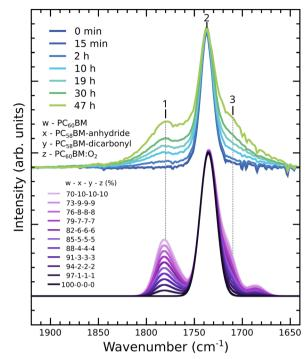
Fig. 7 Experimental IR spectra in the carbonyl region of unexposed PC<sub>60</sub>BM and PC<sub>60</sub>BM exposed to light in air for different exposure times (upper part) compared to calculated spectra with different weighted averages between pristine PC<sub>60</sub>BM, PC<sub>58</sub>BM-anhydride, PC<sub>58</sub>BMdicarbonyl, and PC<sub>60</sub>BM:O<sub>2</sub> (lower part).
