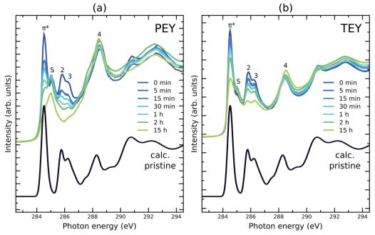
Fig. 2 C1s NEXAFS spectra in (a) partial electron yield (PEY) mode, and (b) total electron yield (TEY) mode of pristine PC<sub>60</sub>BM and PC<sub>60</sub>BM exposed to light in air for different durations, shown in comparison to the calculated NEXAFS spectrum of pristine PC60BM (black line).
