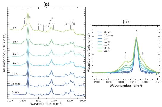
Fig. 4 FTIR absorption spectra of PC<sub>60</sub>BM thin films exposed to light in air for different exposure times (a) in the  $1000-2000 \text{ cm}^{-1}$  region, and (b) zoomed in to the spectral region around the carbonyl peak.
