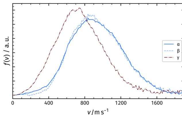
Fig. 7 Velocity distributions for recombinatively-desorbing oxygen from Rh(111) at different desorption temperatures. The desorption of the  $\gamma$ -peak is significantly shifted towards lower velocities compared to the  $\alpha$ -peak and the  $\beta$ -peak.
