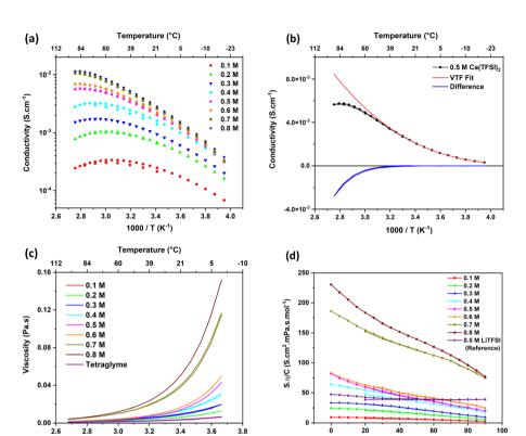
Fig. 1 (a) Temperature dependence of the conductivity of Ca(TFSI)<sub>2</sub>/G4 solutions at different salt concentrations. (b) VTF fit of the conductivity recorded on a 0.5 M Ca(TFSI)<sub>2</sub>/G4 solution. (c) Temperature dependence of the viscosity of Ca(TFSI)<sub>2</sub>/G4 solutions at different salt concentrations. (d) Walden plot of Ca(TFSI)<sub>2</sub>/G4 solutions at different salt concentrations. The Walden plot of a 0.5 M LiTFSI/G4 solution was plotted as a reference for comparison
