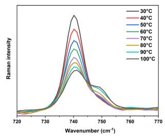
Fig. 5 Evolution in the position and the intensity of the characteristic expansion-contraction mode of TFSI- at 740 cm-1 during the temperature-dependent in situ Raman measurement performed on a 0.1 M Ca(TFSI)<sub>2</sub>/G4 solution.
