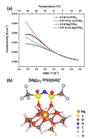
**Fig. 6** (a) Temperature dependence of the conductivity of 0.5 M Mg(TFSI)<sub>2</sub>/G4 solution compared to 0.5 M Ca(TFSI)<sub>2</sub>/G4. A divergence from the VTF model was observed for both solutions. (b) Structure of the [Mg( $\mu_2$ -TFSI)(G4)]<sup>+</sup> ion-pair optimised by the SCAN-rVV10 functional embedded in the VASP code.
