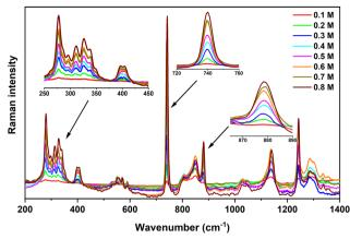
Fig. 4 Raman spectra acquired on Ca(TFSI)<sub>2</sub>/G4 solutions at different salt concentrations. Insets focus on the zoom of some important vibrational modes
