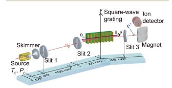
Fig. 2 Schematic of the experimental setup used for reflection of He molecular beams from square-wave gratings. The illustration shows the definitions of the incidence angle  $\theta_{in}$  and detection angle  $\theta$ .
