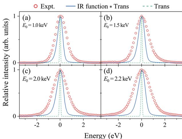
Fig. 3 Energy spectra of H<sub>2</sub> obtained at  $E_0 =$  (a) 1.0, (b) 1.5, (c) 2.0, and (d) 2.2 keV, respectively. The solid lines are the associated practical instrumental response (IR) functions (IR function  $\times$  Trans). The dashed lines are the calculated Doppler broadening due to molecular translational motion.
