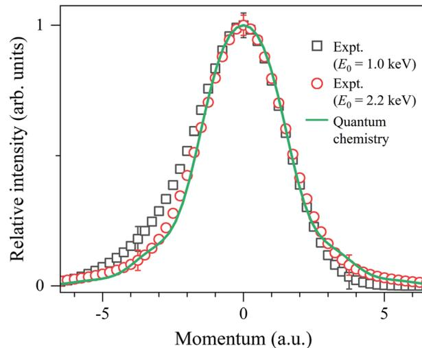
Fig. 4 Comparison between experimental Compton profiles of H<sub>2</sub> measured at  $E_0 = 1.0$  and 2.2 keV. The solid line represents the associated theoretical profile at  $K = \infty$ .
